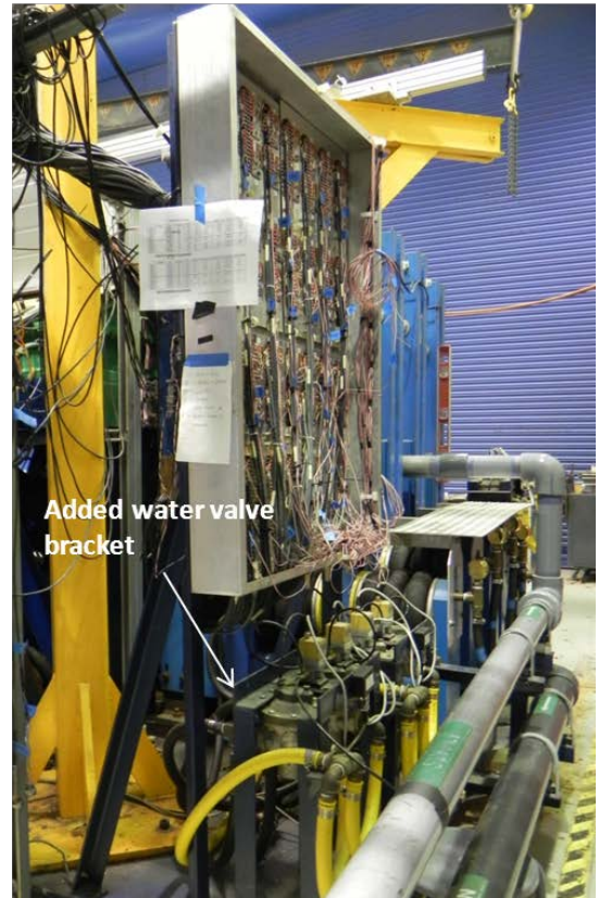
Figure 2. Photographs of Strain Gage Completion Bridge Board Relocation
