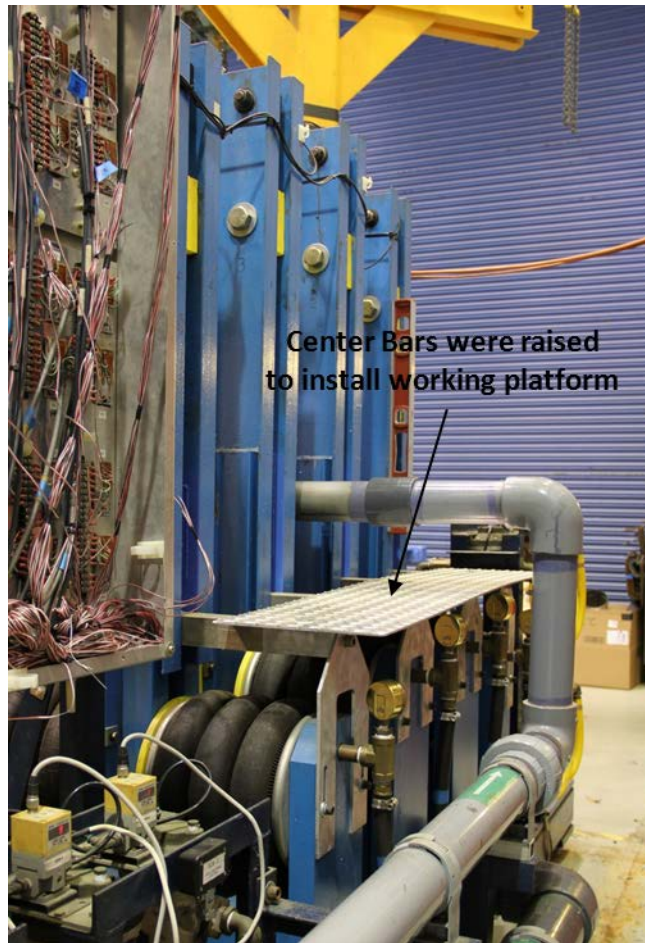
Figure 10. Photo of Guide Rail Assembly Final Configuration
