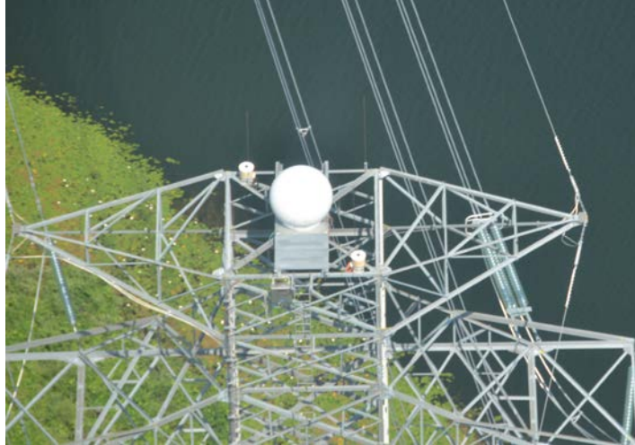
Figure 4. DeTect X-Band ADLS Radar With Radome Enclosure
