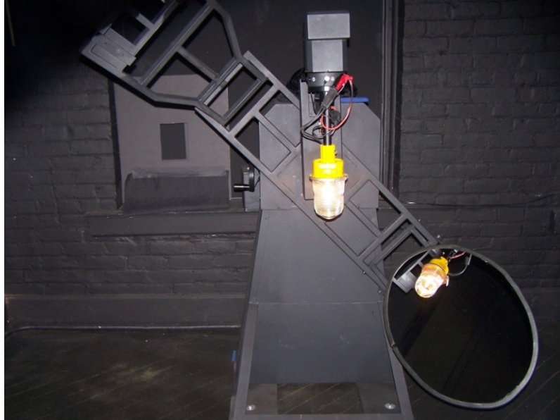
Figure 1. View of a luminaire under test mounted on the type-C mirror goniophotometer. The geometric center of the luminaire was used as reference for alignment.
