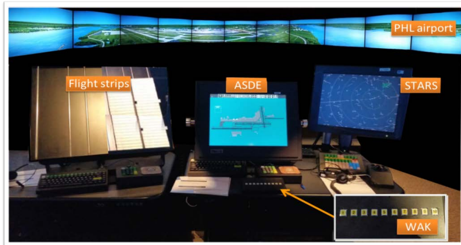
Figure 4. Tower Simulator Hardware
