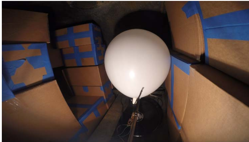
Figure 6. Balloon rig in pressure chamber immediately prior to ignition
