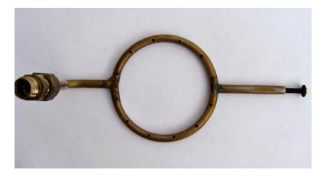
Figure 1. Exhaust gas sampling ring
