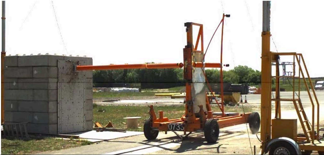
Photo: Impact Testing of Approach Light System (ALS) Tower at MIRA Ltd Facility in the United Kingdom
