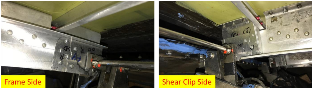
Figure 61. Configuration of frame repair from both ends
