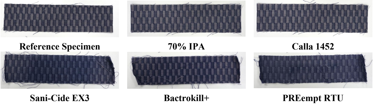
Figure 64. Color qualitative comparison with submersion method – Lantal
