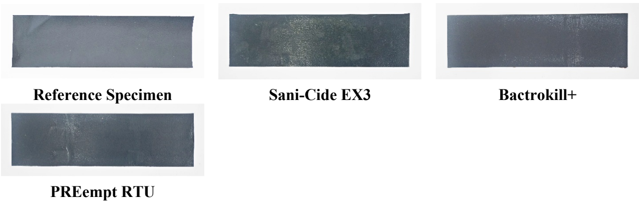
Figure 102. Color qualitative comparison with wiping method – Perrone Feather Weight
