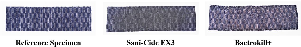
Figure 103. Color qualitative comparison with wiping method – Lantal
