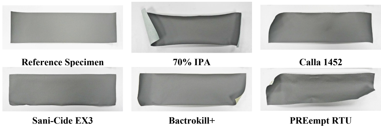
Figure 56. Color qualitative comparison with submersion method – E-Leather CL820 front face
