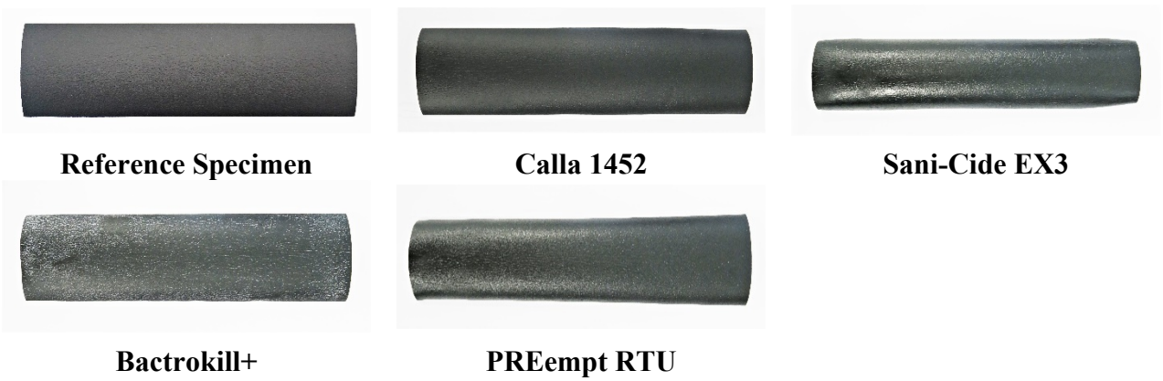
Figure 96. Color qualitative comparison with wiping method – Ultrafabrics 492-6579FR12 front face
