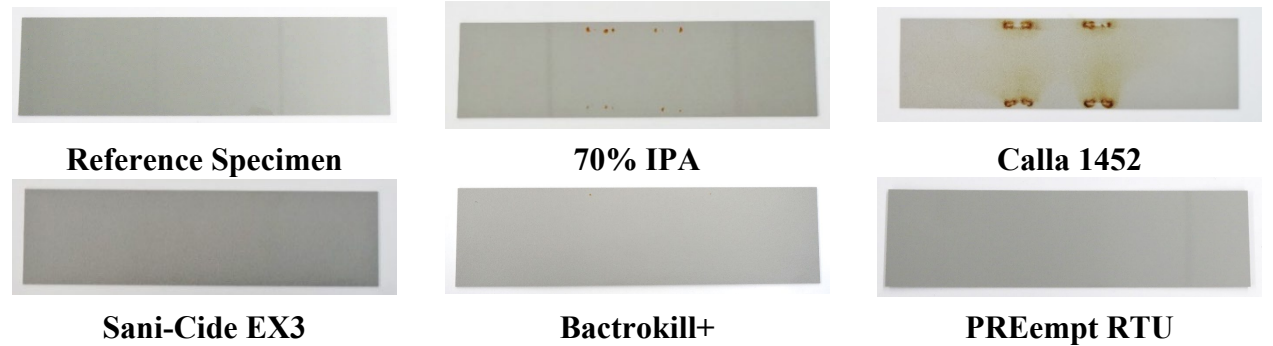
Figure 51. Color qualitative comparison with submersion method – Lexan XHR shade 1
