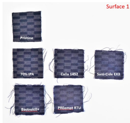
Figure 85. Color measurement results – Ultraleather ULFRB971-1363 back face
