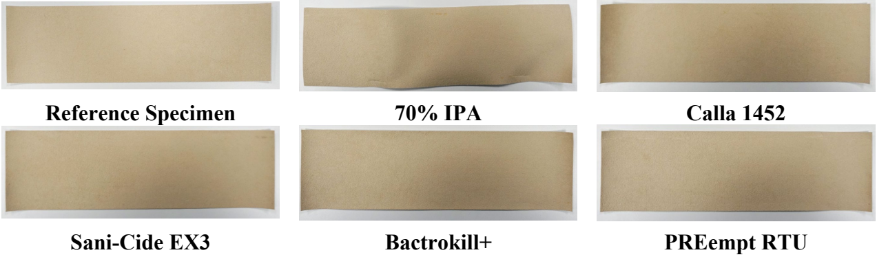
Figure 61. Color qualitative comparison with submersion method – Tapisuede TSFRC0961 back face
