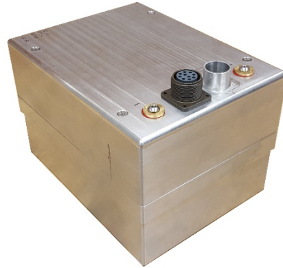
Figure 25. Fully 26 V, 20 Ah prototype Li-ion battery with packaging technology and BMS
