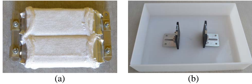
Figure 8. Nail-penetration abuse and failure propagation test setup; (a) 1S4P NMC cell pack with 2 mm knit cell jackets, and (b) nail penetration test basin
