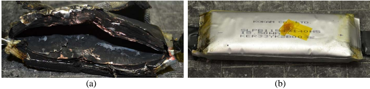
Figure 32. Cell pack tear-down after mechanical abuse and failure propagation test for a 1S4P cell pack with 1 mm thick packaging materials: (a) failed cell with electrode compression damage due to over penetration of the nail and (b) surviving cell exhibiting swelling but no venting
