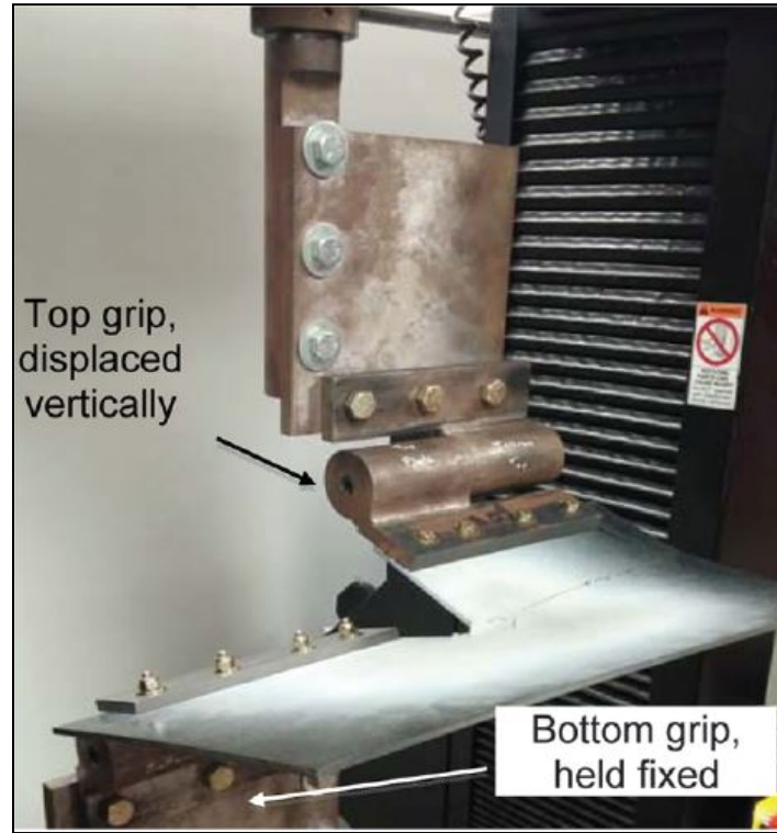
Figure 5. Image of specimen in loading configuration
