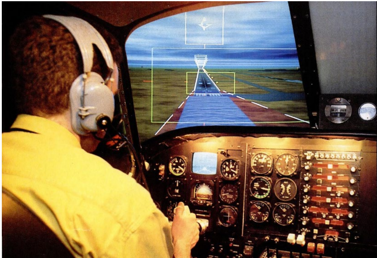
Figure 5. Simulator with EZ-Fly controls and highway in the sky heads-up display
