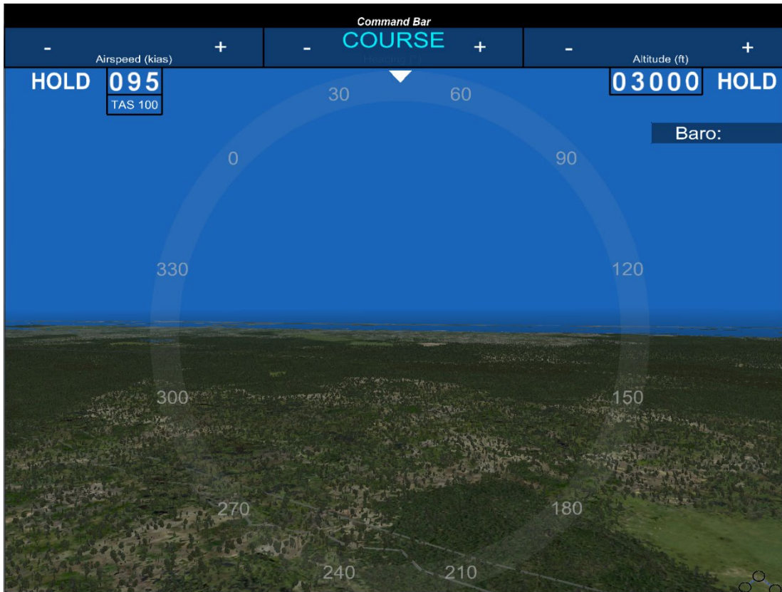
Figure 2. Forward display while holding a course
