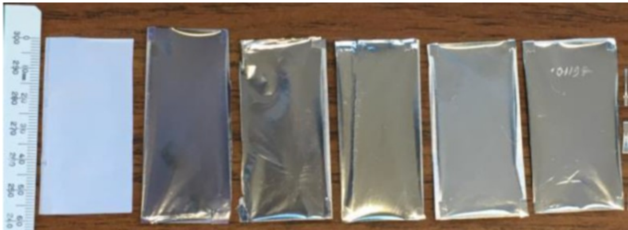
Figure 38. PE coated with different thickness of Ag (from left to right – pristine PE, 6 nm, 12 nm, 18 nm, 24 nm, and 30 nm Ag on PE) for dendrite sensing
