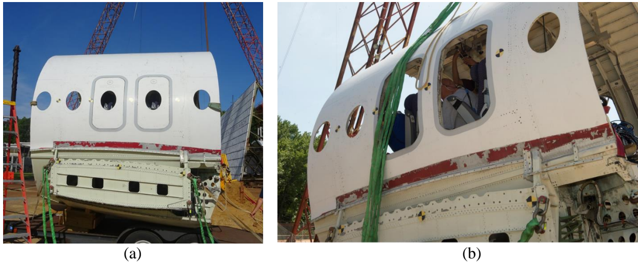
Figure 5.8. Wingbox section port emergency exit doors pre-test (a) and removed post-test (b)
