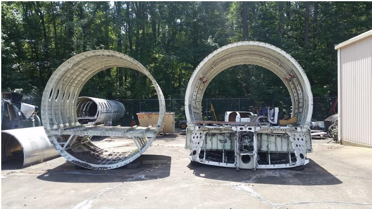
Figure 2.2. Unmodified F28 test article sections—forward (left), and wingbox (right)
