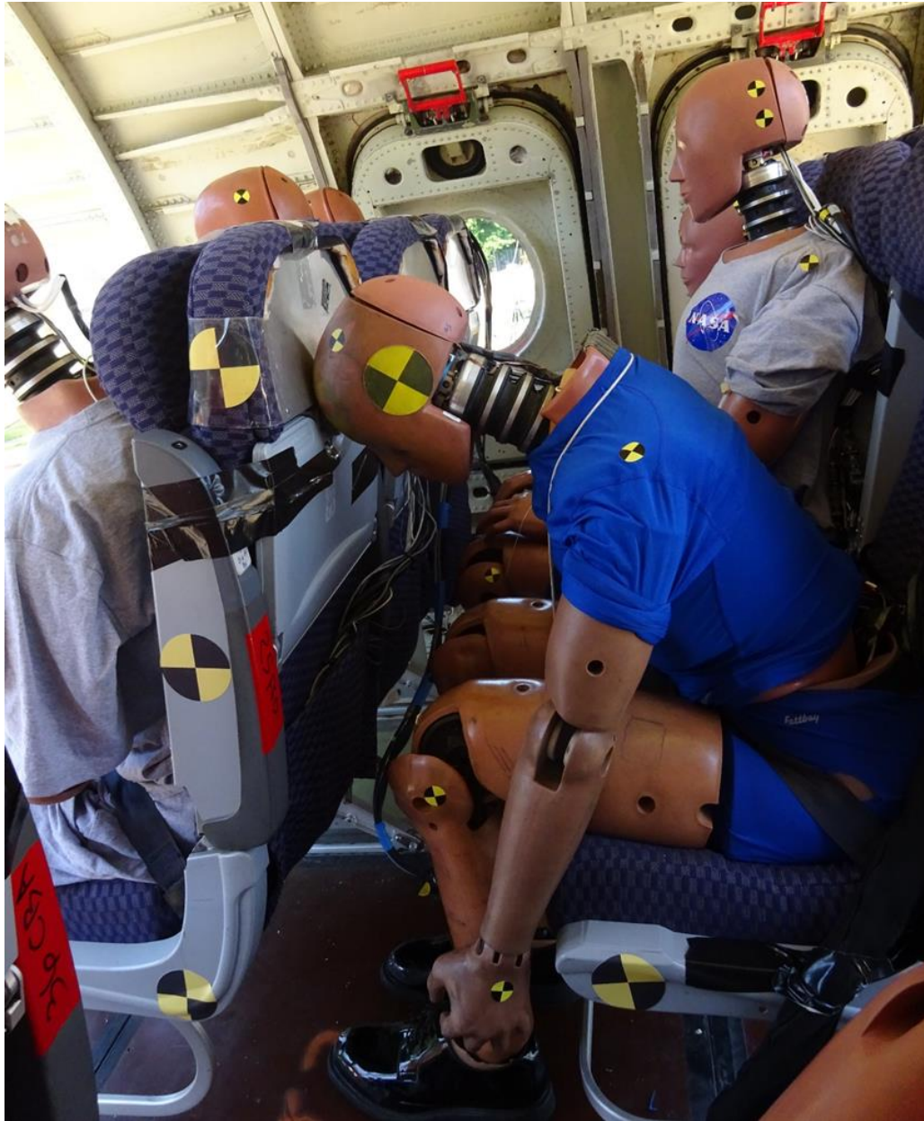
Figure 5.24. ATD 3 in the brace position
