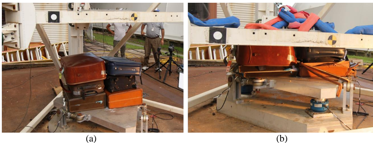
Figure 4.5. Luggage test 2 pre-test (a) and post-test (b)
