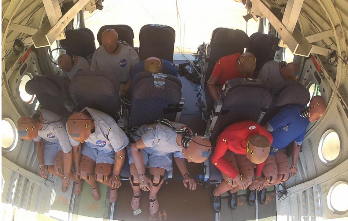
Figure 5.25. Wingbox section post-test ATD positions
