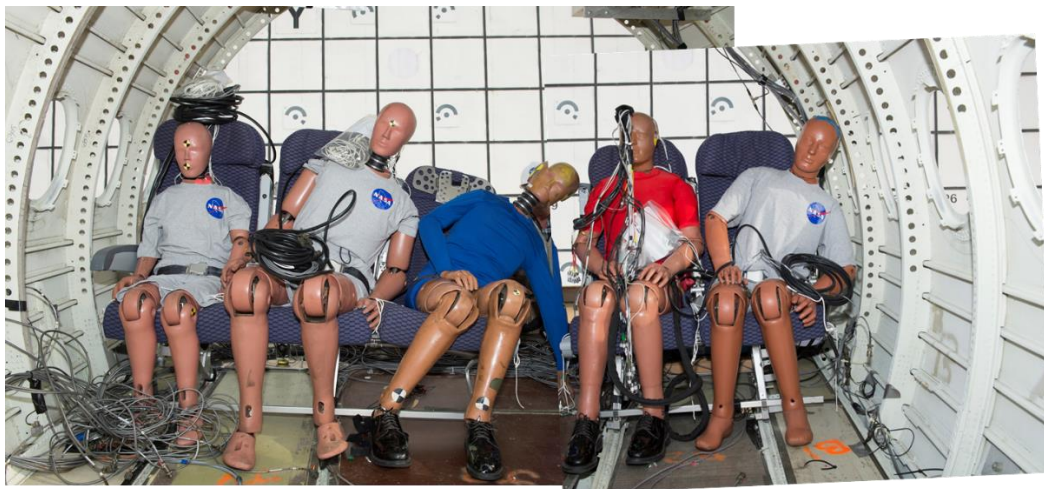
Figure 3.20. Forward section rear row ATDs (Seats 1 through 5)
