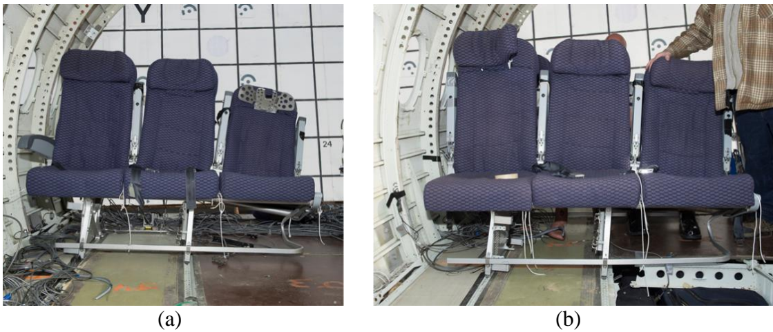
Figure 3.24. Post-test triple seats—rear (a) and front (b)
