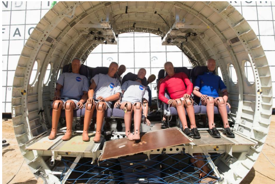
Figure 3.19. Forward section front row ATDs (Seats 6 through 10)
