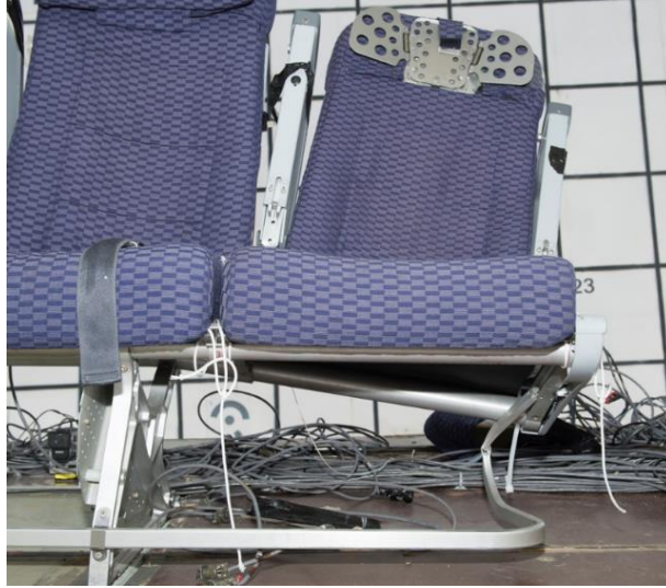
Figure 3.25. Post-test rear triple aisle seat deformation (seat 3)
