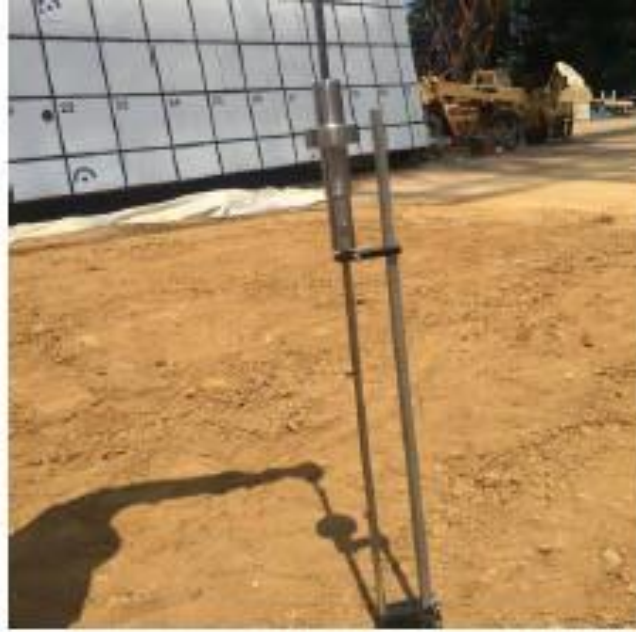
Figure 10. Photograph and schematic of the DCP
