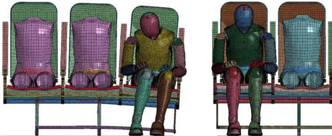
Figure 26. Deformation of a single row of seats with two LSTC-detailed FEM occupant models and three rigid torso models
