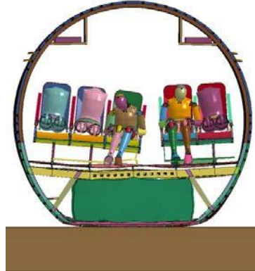
Figure 41. Forward section FEM with ATDs and seats - deformation sequence
