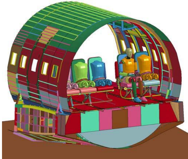
Figure 65. Wing-box section model with seats and ATD models
