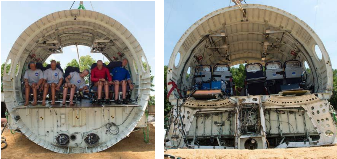
Figure 51. Two post-test photographs of the F-28 wing-box section: (a) front view and (b) rear view
