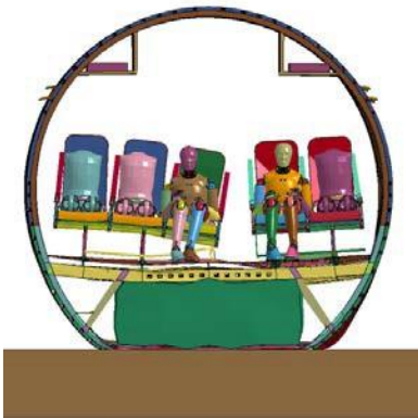
Figure 41. Forward section FEM with ATDs and seats - deformation sequence
