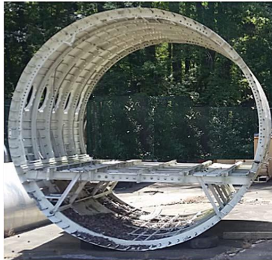
Figure 3. Photograph of the unloaded F-28 forward fuselage section
