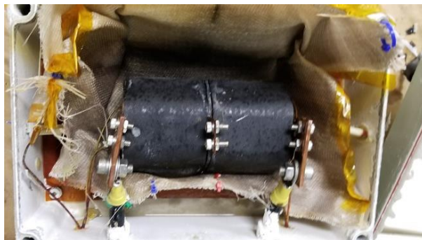
Figure 59. Evidence of venting, but no fire in RF battery from external short
