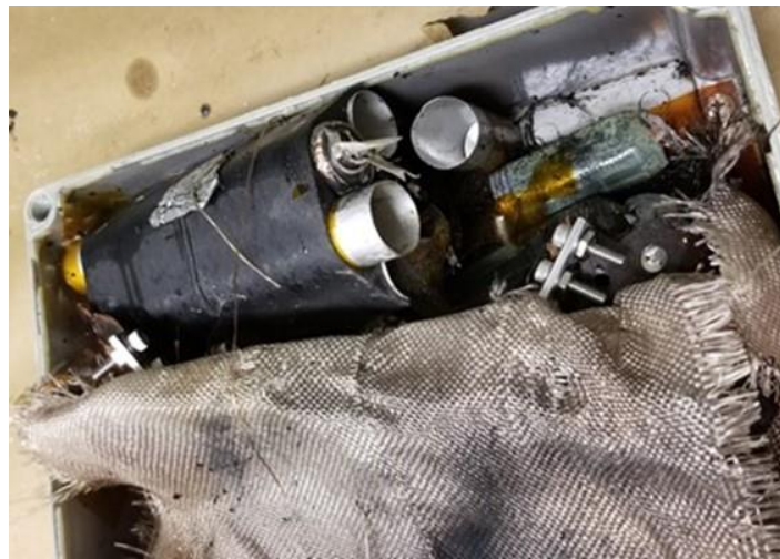
Figure 54. Evidence of venting, but no fire, in overcharge test of BL module
