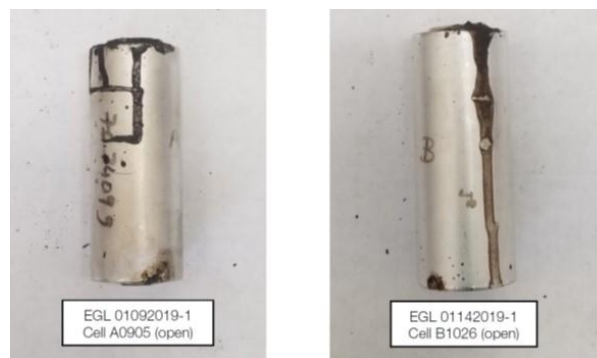
Figure 27. RF (left) & BL (right) cells at the end of open ARC tests, indicating cell venting
