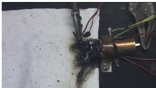
Figure 21. Paper towel coated with flame-retardant paint did not burn, despite the complete burning of the LFP cell during thermal runaway in the overcharge test
