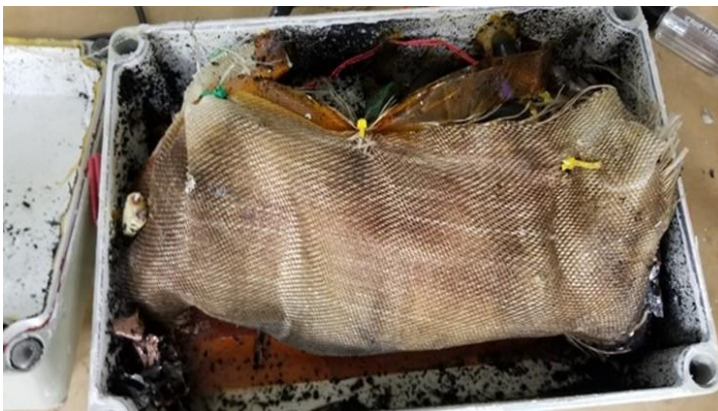
Figure 64. RF battery showed half of the cells intact and no evidence of fire
