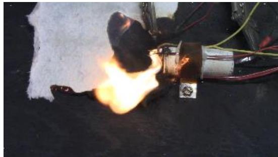
Figure 20. Flame-retardant painted LFP cell placed on an uncoated paper towel did not prevent flame propagation in the overcharge test
