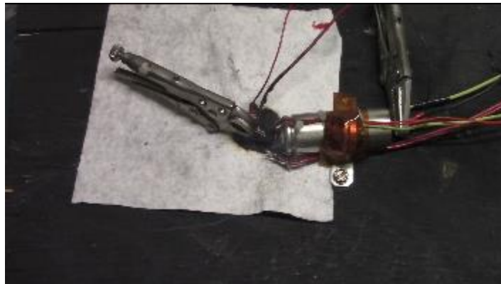
Figure 18. Paper towel coated with FR-A did not burn, but had a localized charring when the cell went into thermal runaway in the overcharge test
