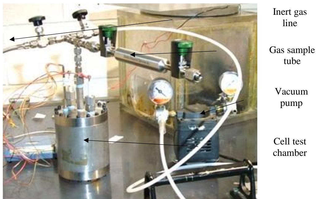
Figure 22. Setup for off-gas sampling test
