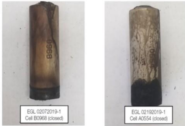
Figure 30. RF (right) and BL (left) cells at the end of closed ARC tests, showing profuse cell venting
