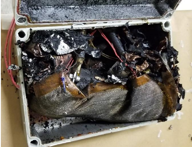
Figure 63. BL battery showed 13 cells venting and burning in overheating test
