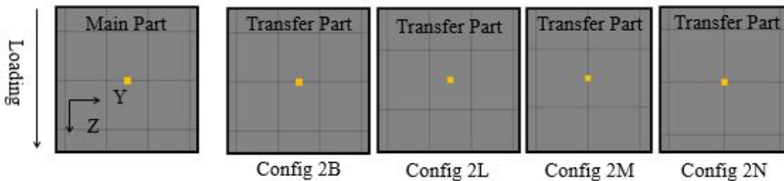
Figure 67. Contact points on main part vs. transfer part for analysis of mesh-independent spotweld beam SJMs
