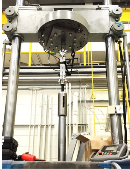
Figure 21. High-rate servo hydraulic MTS testing machine at NIAR
