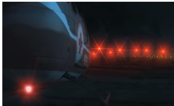
Figure 4.20: An OCAS System Illuminating a Wind Turbine Farm for a Helicopter 31
