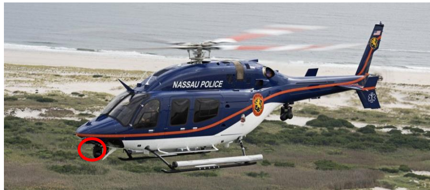
Figure 8.2: Camera Obstructing Lower Wire Cutter on the Bell 429 56
