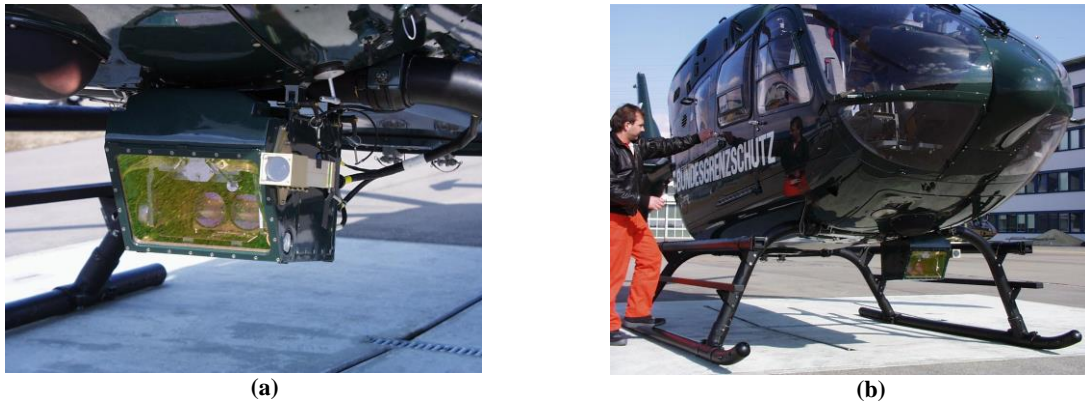
Figure 4.13: HELLAS on EC 135 (Schulz, Scherbarth, & Fabry, 2002)
