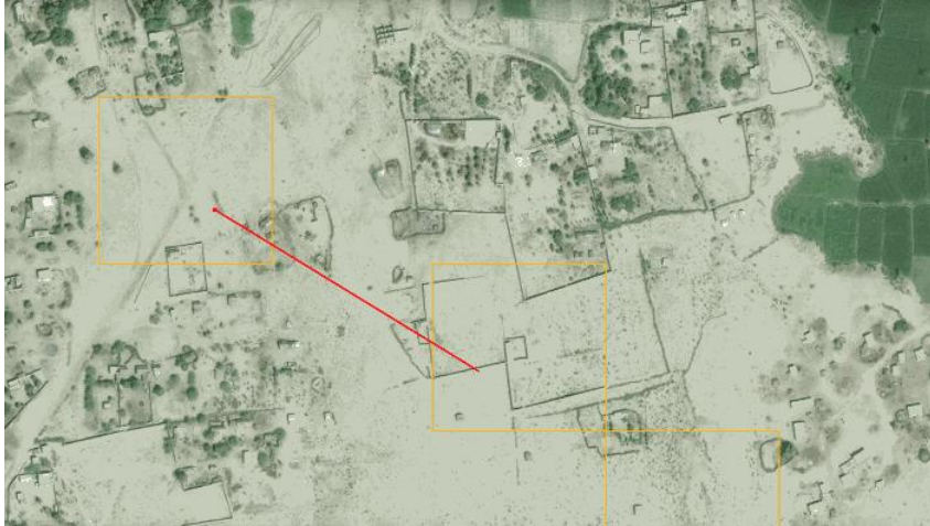
Figure 2.10: ML Algorithm Prediction of HV Tower Locations 9
