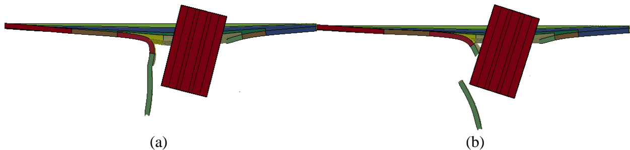
Figure 24. Snapshots of two ballistic impact simulations at 0.5 msec: (a) 20° oblique angle and (b) 25° oblique angle
