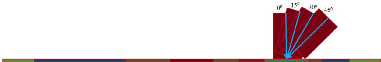
Figure 19. Overlap of ballistic impact setups of the oblique angle variation series (blue arrows indicate the projectile flight direction)
