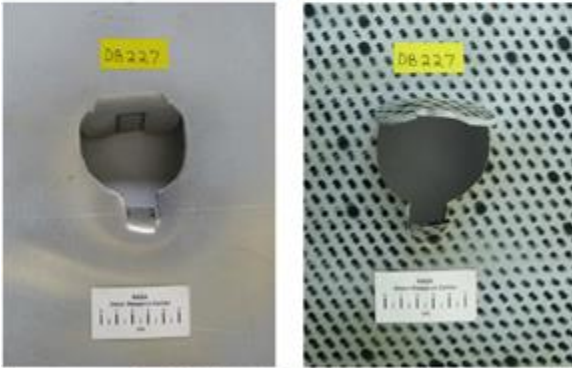
Figure A120 -- Front (left) and back side views of impacted panel in test DB227.
