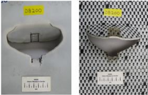
Figure A11 — Front (left) and back side views of impacted panel in test DB200
