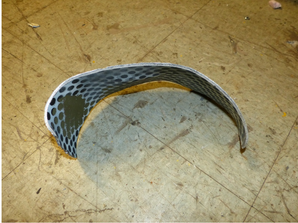
Figure D.15.—LG1113 ejected material from panel.
