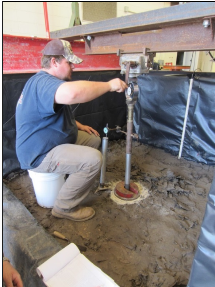
Figure 15. The CBR Testing on the CH Subgrade
