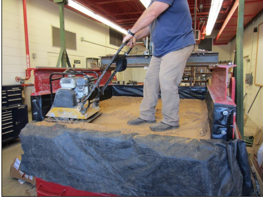
Figure 17. Compaction of Subbase Material
