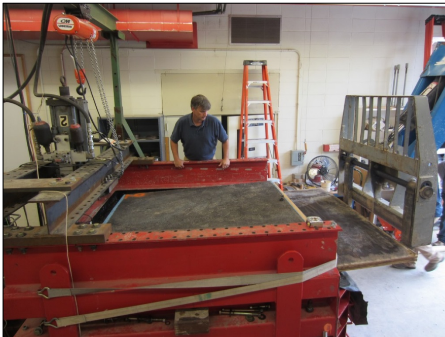
Figure 31. Placement of HMA on Top of Base Course
