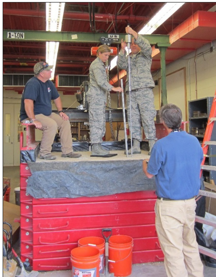
Figure 22. The DCP Testing at the Surface of the Base Course
