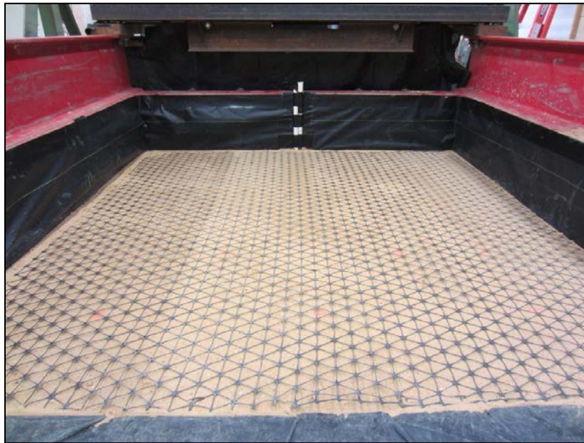
Figure 19. Prepared Surface Prior to Placement of Crushed Limestone Materials
