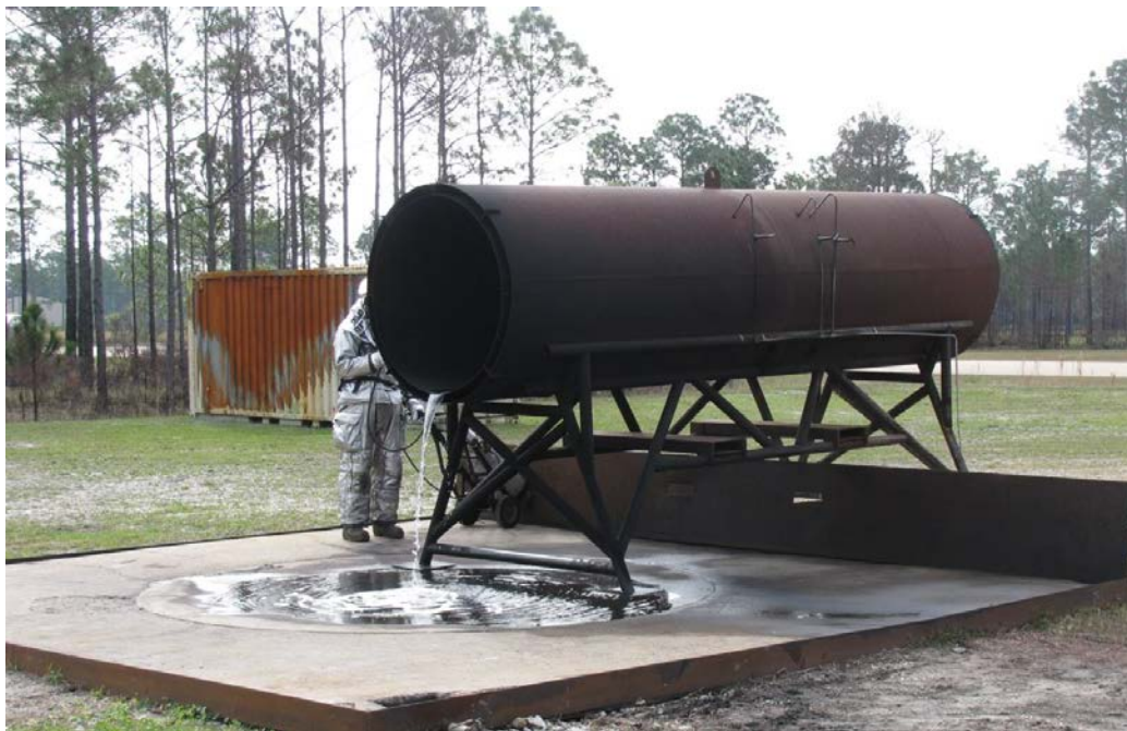
Figure 16. Simulated Engine Nacelle Running Fuel Fire Test Apparatus
