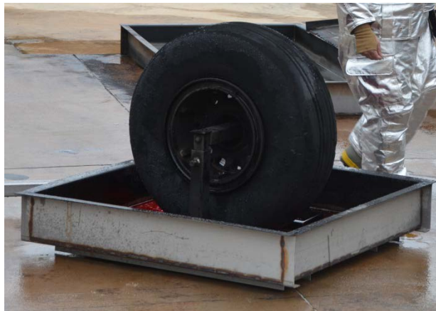
Figure 9. Simulated Wheel Brake Fire Involving Hydraulic Fluid Test Setup
