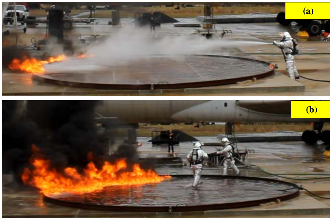
Figure 21. Test 1: Novec 1230 30-ft Pan Fire
