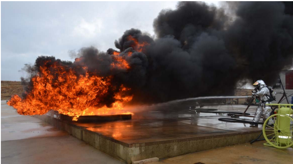
Figure 19. Novec 1230 Three-Dimensional Inclined-Plane Fire Test 4
