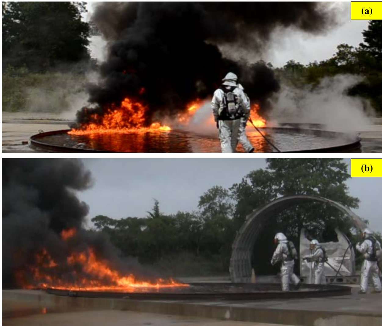
Figure 24. Test 1: Halotron I 30-ft Pan Fire
