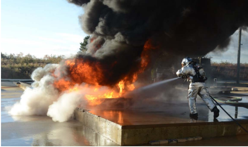
Figure 20. Halotron I Three-Dimensional Inclined-Plane Fire Test 4
