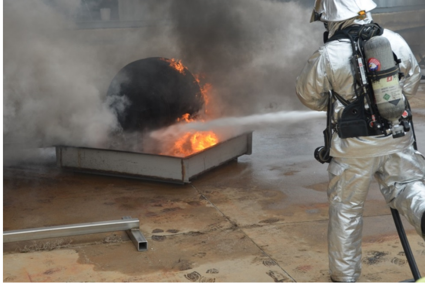
Figure 18. Approach Path for Simulated Wheel Brake Fire Involving Hydraulic Fluid Test
