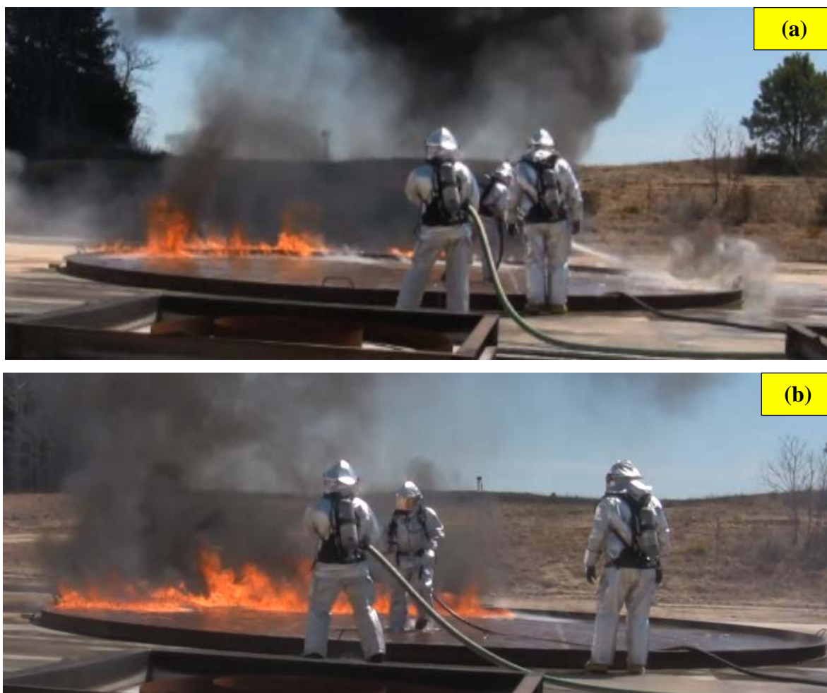
Figure 22. Test 2: Novec 1230 30-ft Pan Fire
