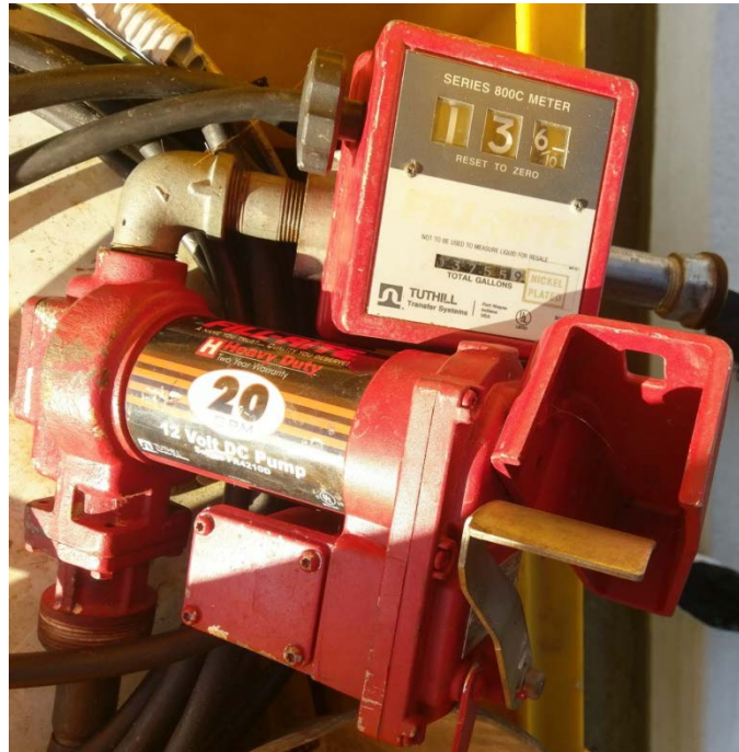
Figure 6. Fill-Rite FR4211D Fuel Pump With a Tuthill 800C Flow Meter
