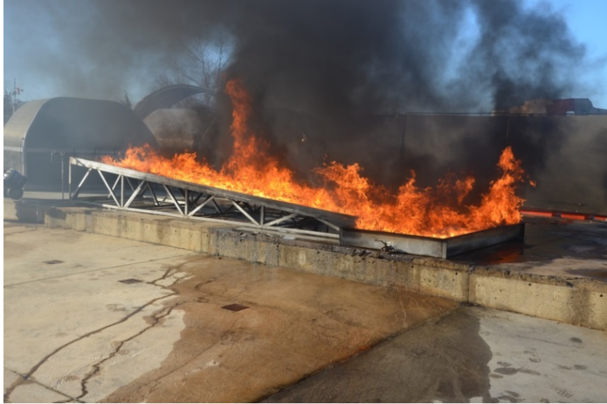
Figure 12. Three-Dimensional Inclined-Plane Fire Test During Preburn
