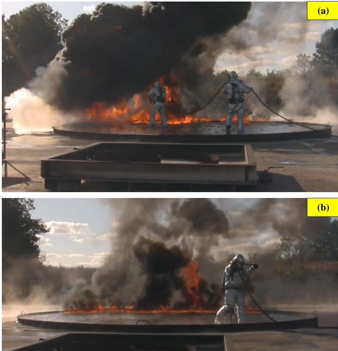
Figure 26. Test 3: Halotron I 30-ft Pan Fire
