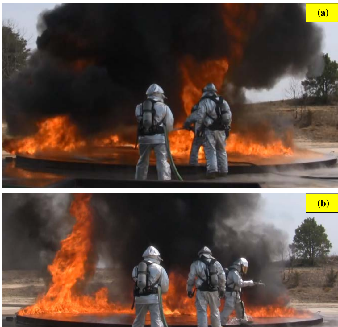
Figure 23. Test 3: Novec 1230 30-ft Pan Fire
