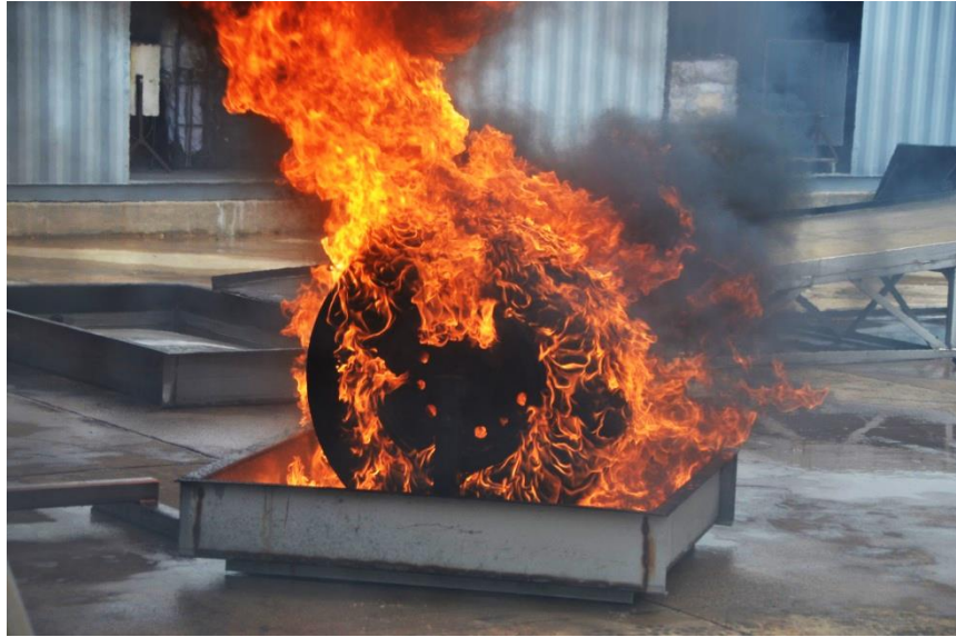
Figure 10. Fully Involved Simulated Wheel Brake Involving Hydraulic Fluid Test Fire
