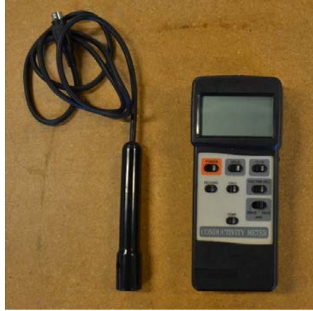
Figure 5. Traceable 4169 Dual-Display Conductivity Meter
