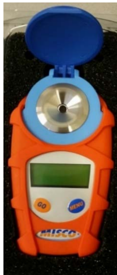
Figure 4. Misco PA202 Refractometer
