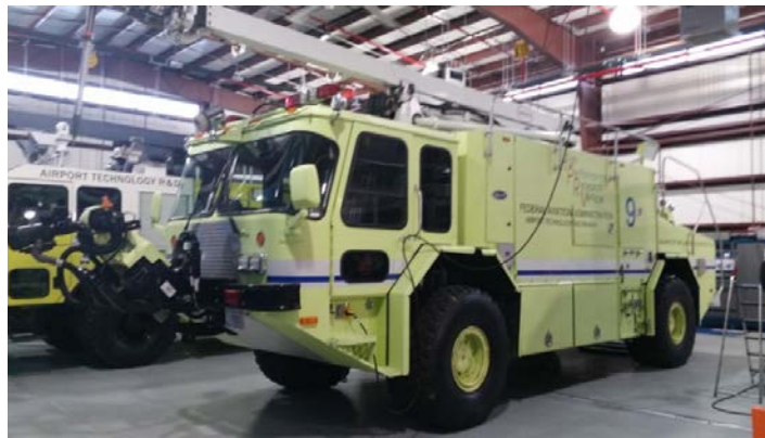
Figure 2. The 1992 E-ONE Titan 4x4 FAA ARFF Research Vehicle “Crash 9”
