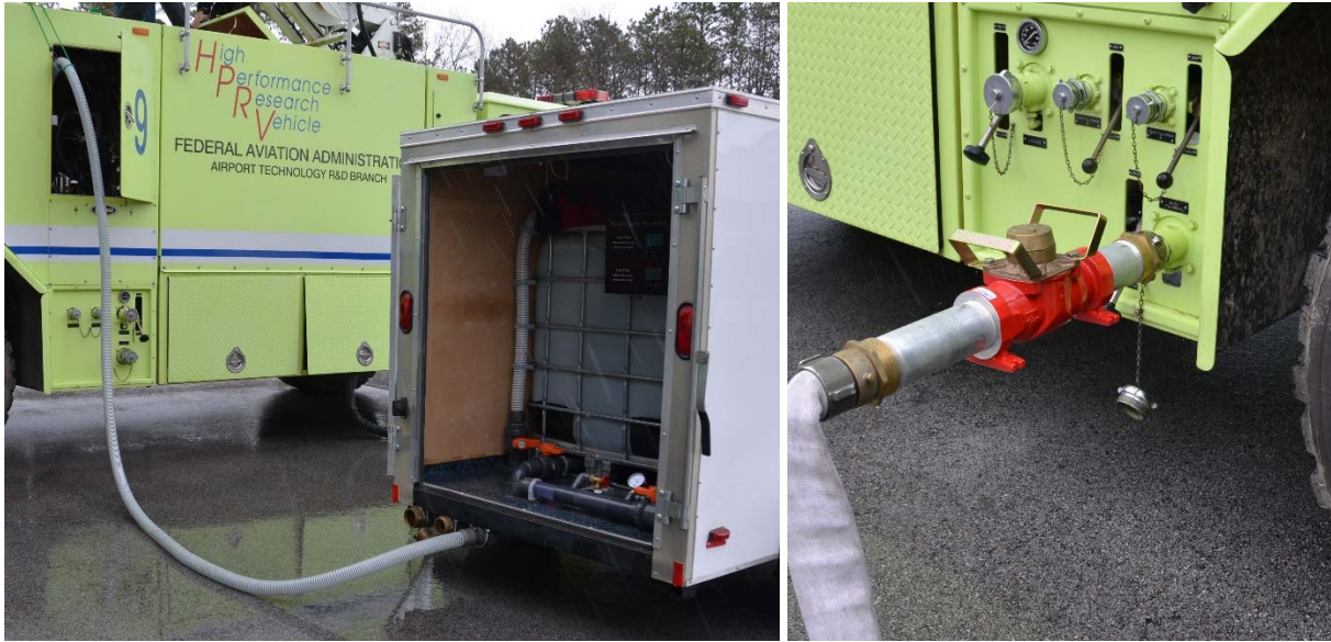
Figure 13. NoFoam System Connections on Crash 9
