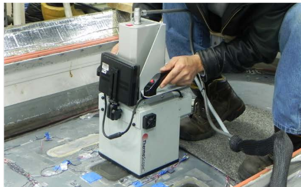
Figure 27. (a) TWI ThermoScope® II high-performance PC system complete with MOSAIQ® analysis software, and (b) TWI ThermoScope® II integrated illumination head
