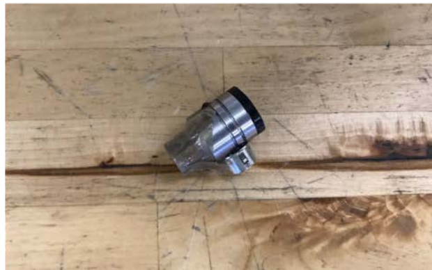
Figure J-1. (a) Olympus BondMaster 1000e+, and (b) S-PR-5 - 250 kHz resonance probe
