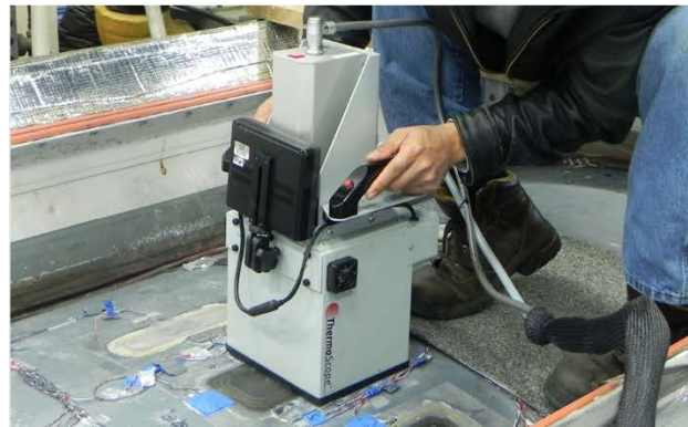
Figure I-1. (a) TWI ThermoScope® II high-performance PC system complete with MOSAIQ® analysis software, and (b) TWI ThermoScope® II integrated illumination head
