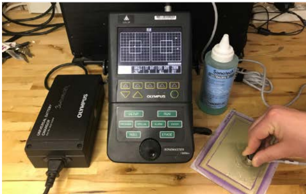
Figure J-1. (a) Olympus BondMaster 1000e+, and (b) S-PR-5 - 250 kHz resonance probe
