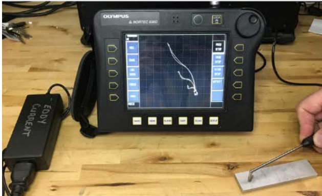
Figure H-3. (a) Portable Eddy Current Flow Detector, (b) PowerLink™ Absolute Shielded Metal Detachable Pencil Probe, and (c) PowerLink™ Standard Bridge Detachable Surface Probe
