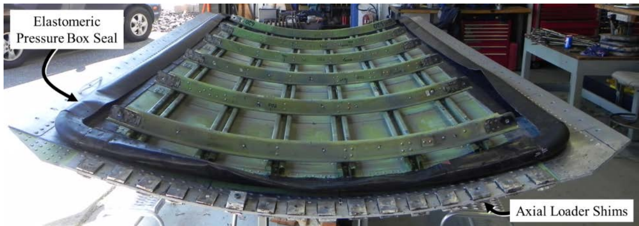
Figure 6. Fuselage panel after installation of elastomeric pressure box seal and axial loader shims
