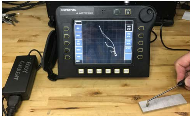
Figure 26. (a) Portable Eddy Current Flaw Detector, (b) PowerLink™ Absolute Shielded Metal Detachable Pencil Probe, and (c) PowerLink™ Standard Bridge Detachable Surface Probe
