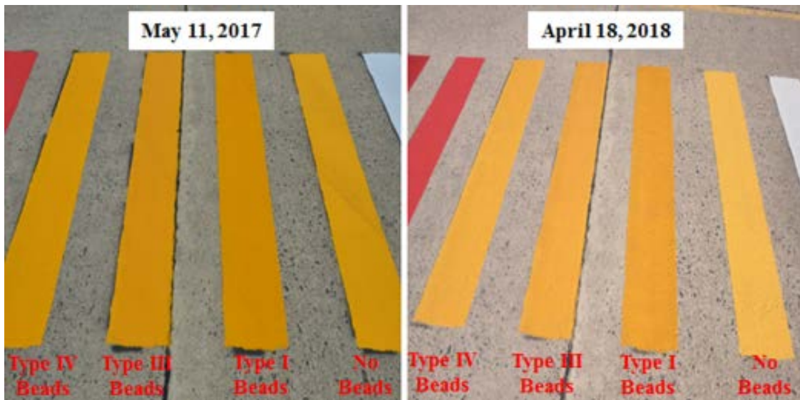
Figure B-14. Yellow Waterborne Type III at ACY—May 2017 (Left) vs April 2018 (Right)
