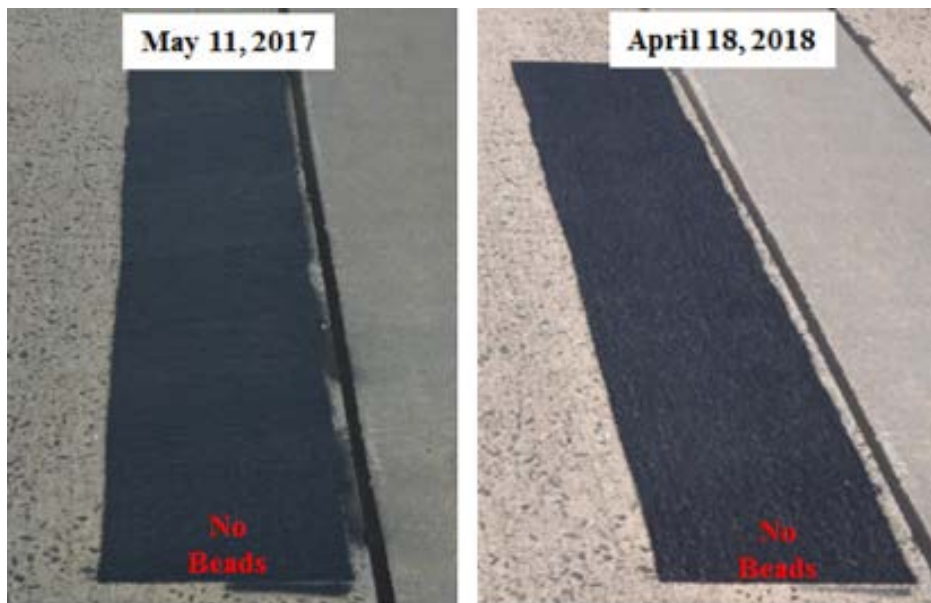
Figure B-4. Black Waterborne Type I at ACY—May 2017 (Left) vs April 2018 (Right)
