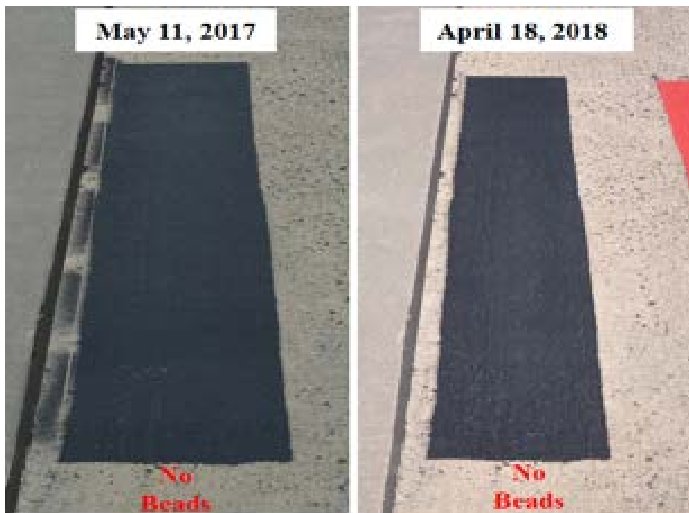
Figure B-16. Black Waterborne Type III at ACY—May 2017 (Left) vs April 2018 (Right)
