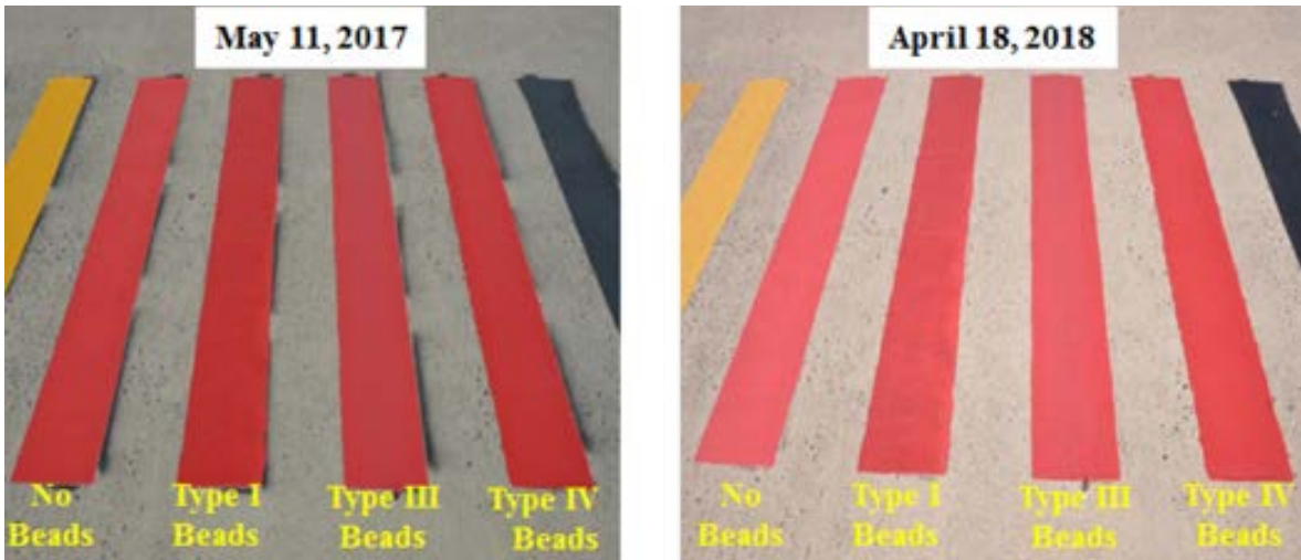
Figure B-7. Red Waterborne Type II at ACY—May 2017 (Left) vs April 2018 (Right)
