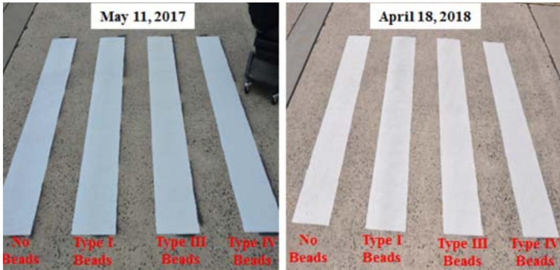
Figure B-13. White Waterborne Type III at ACY—May 2017 (Left) vs April 2018 (Right)
