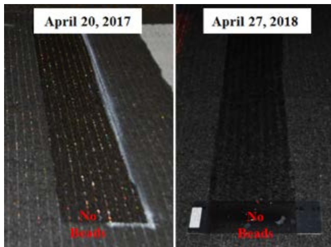
Figure E-4. Black Waterborne Type I at EWR—April 2017 (Left) vs April 2018 (Right)
