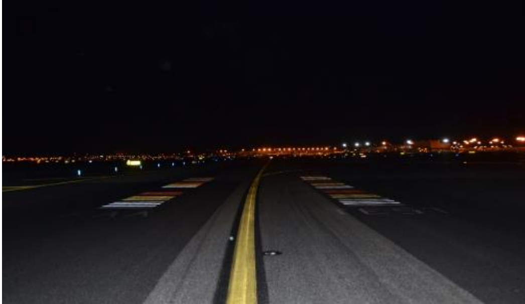
Figure 46. Surface Marking Test Deck on EWR Taxiway N
