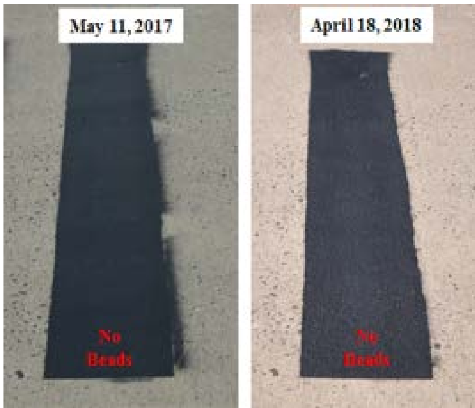
Figure B-8. Black Waterborne Type II at ACY—May 2017 (Left) vs April 2018 (Right)
