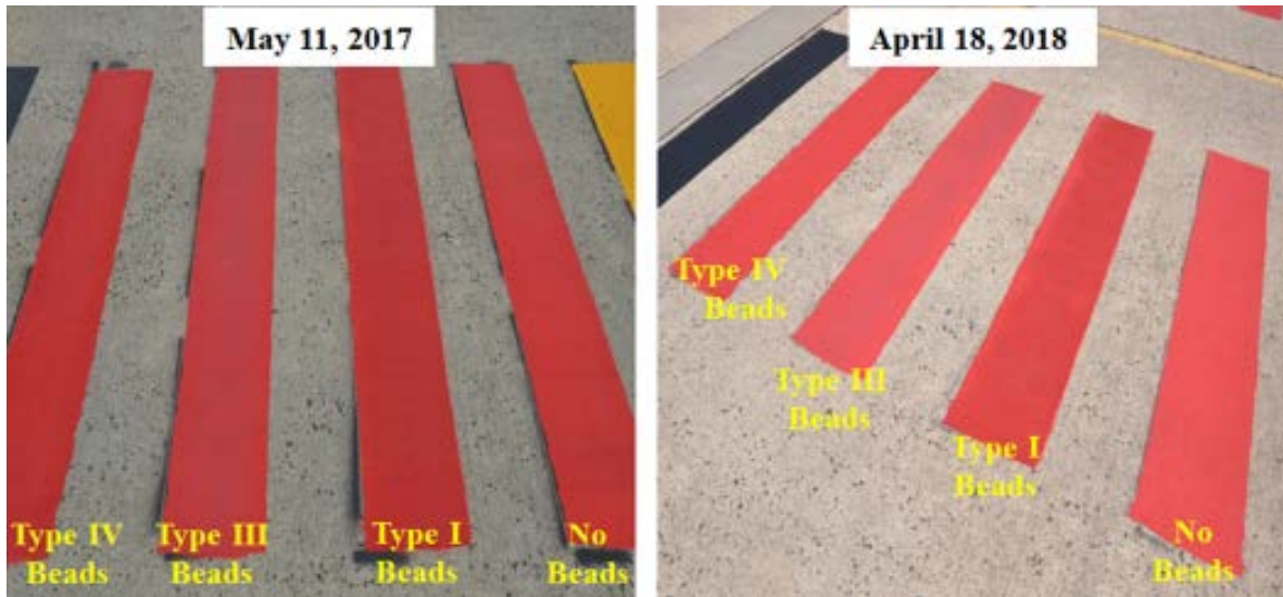
Figure B-15. Red Waterborne Type III at ACY—May 2017 (Left) vs April 2018 (Right)
