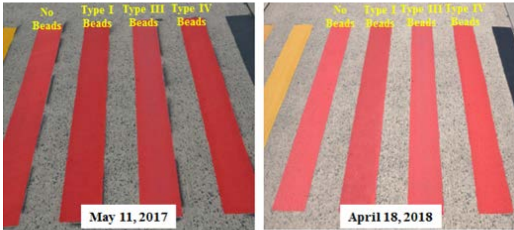
Figure B-3. Red Waterborne Type I at ACY—May 2017 (Left) vs April 2018 (Right)
