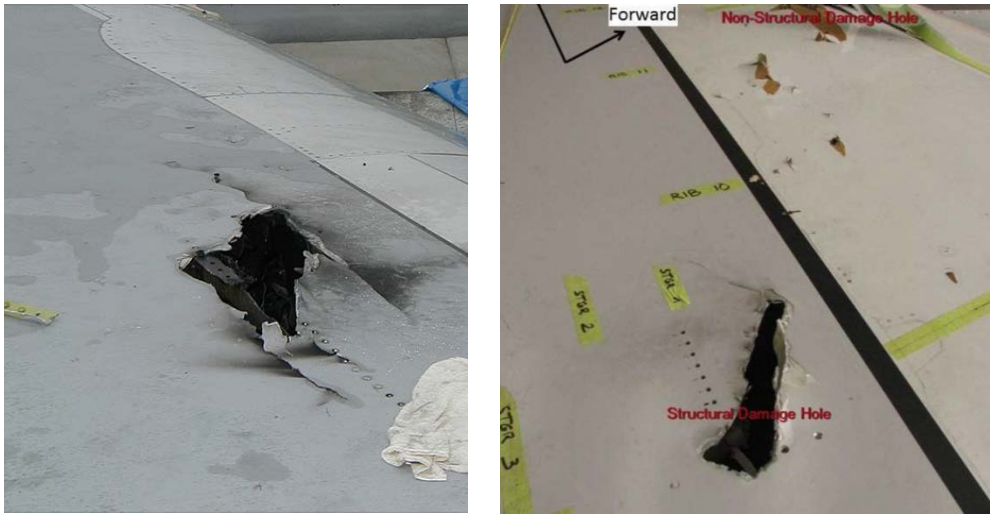
Figure 56. Upper-wing skin damage, HPT disk event
