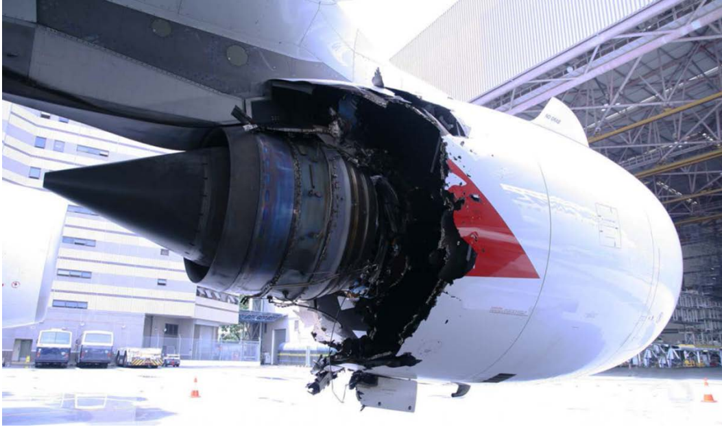
Figure 55. Turbine disk failure
