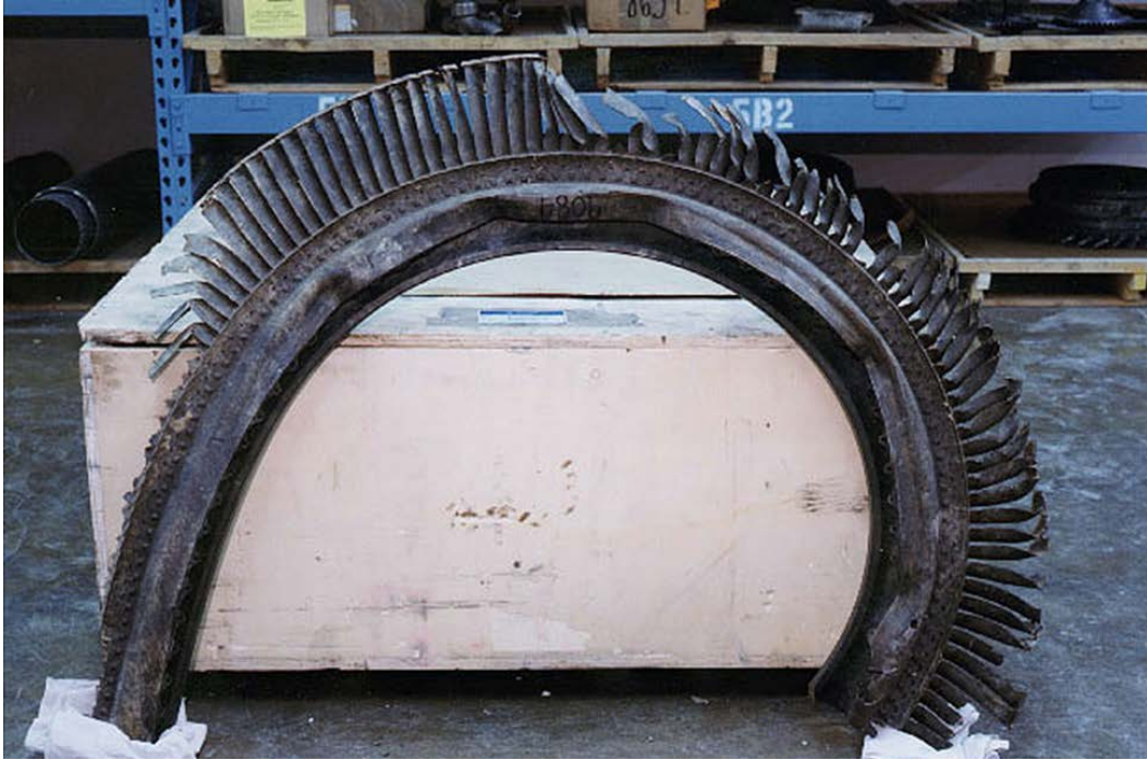
Figure 74. Uncontained LPT disk segment
