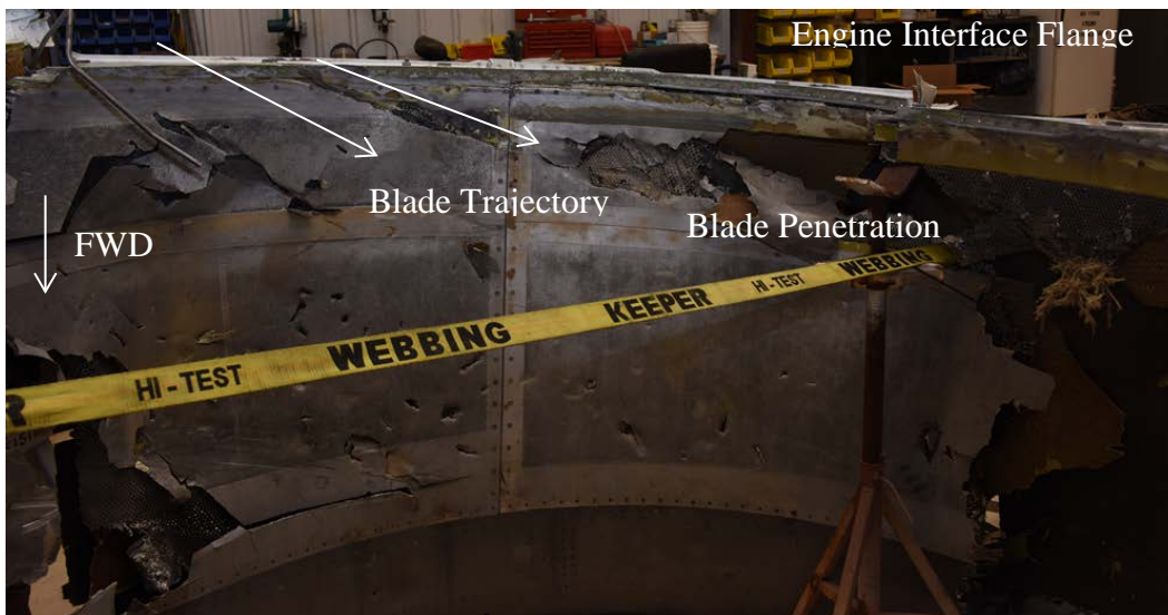
Figure 106. Helical failure trajectory, inlet inner barrel
