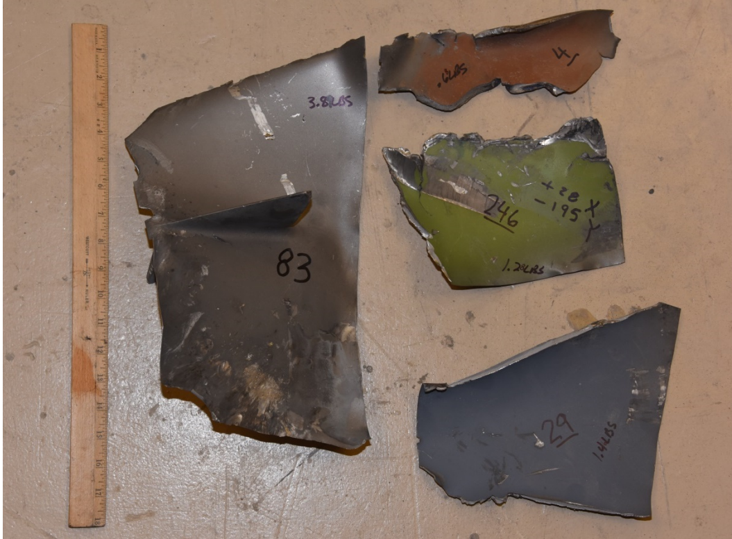
Figure 107. Fan blade fragments from blade-separation event
