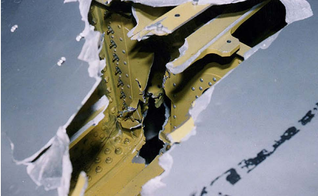
Figure 80. Wing structure damage, LPT disk event
