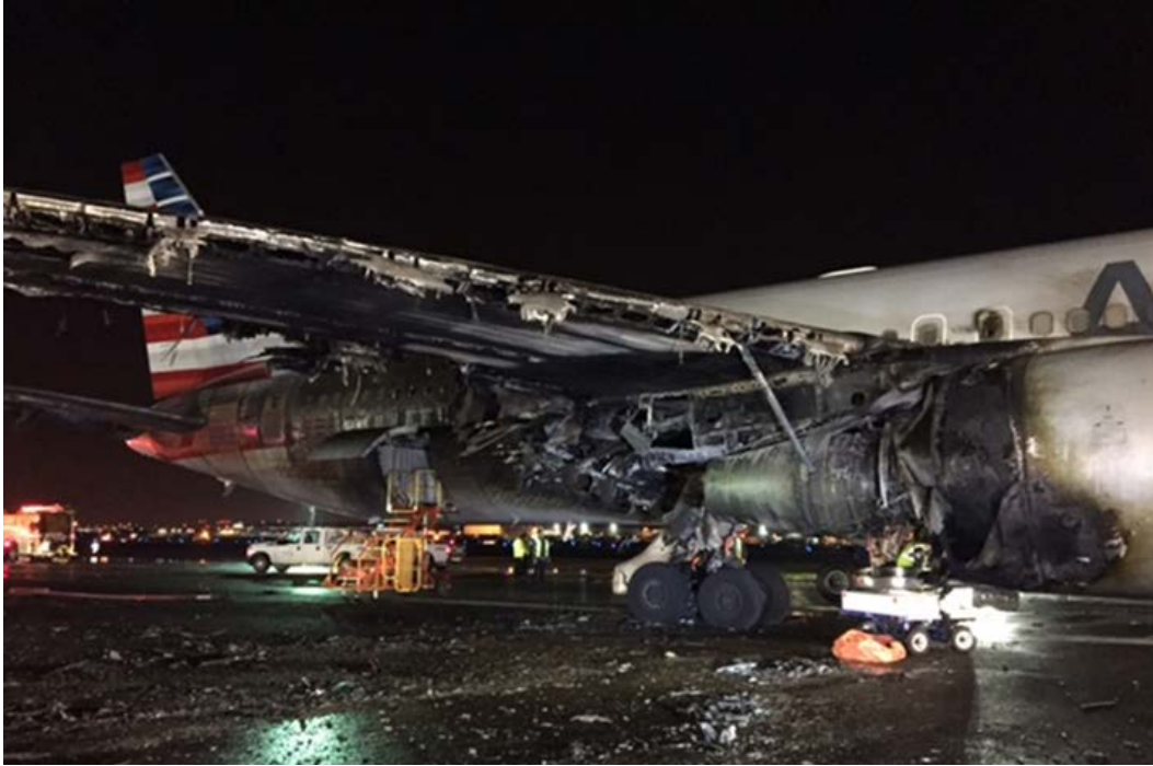
Figure 1. Uncontained turbine disk event
