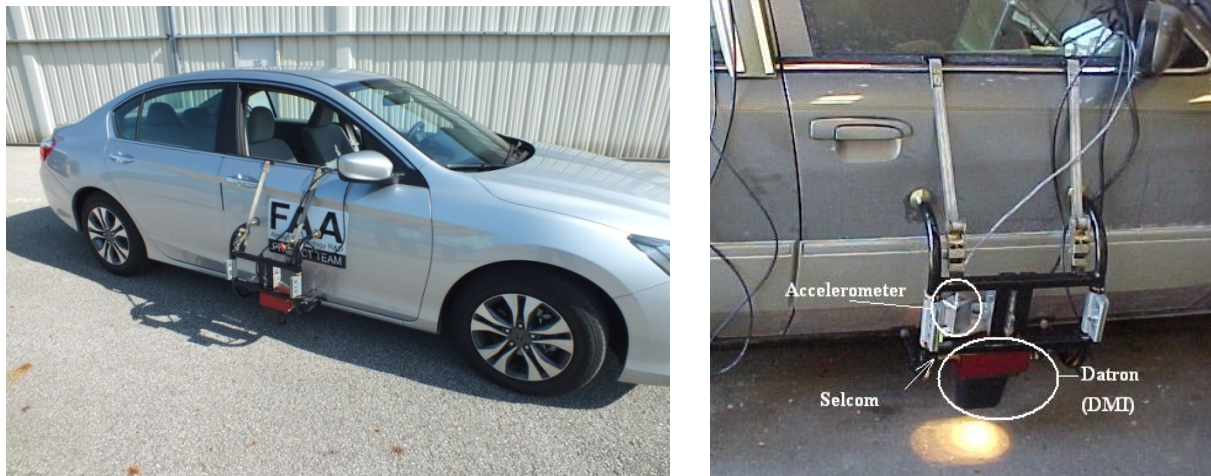
Figure 4. The FAA Surface Profiling Equipment
