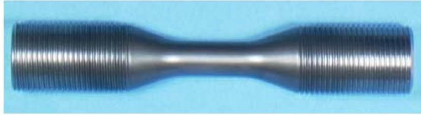
Figure E-16. Cylindrical fatigue specimen containing embedded defect
