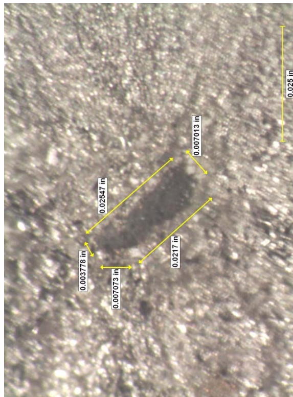
Figure E-19. Inclusion observed on fracture surface of specimen MWF 6114
