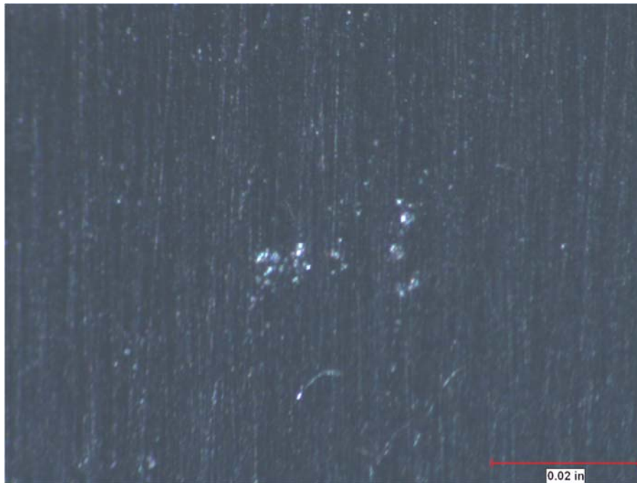
Figure E-17. IN-718 specimen MWF6116 gauge section prior to shot peening
