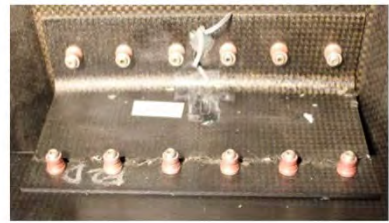
(e) Complete crack along the bolt lines (ST02)
