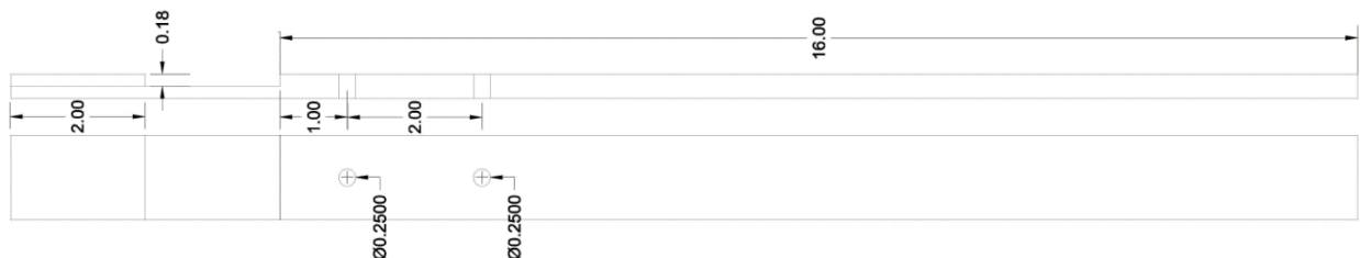
Figure 58. Two-fastener experimental specimen [19]
