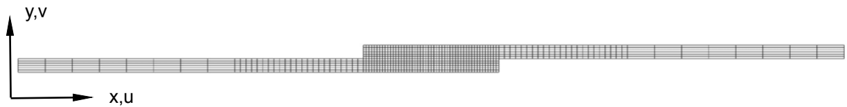
c. Single lap-shear specimen with increased overlap.
