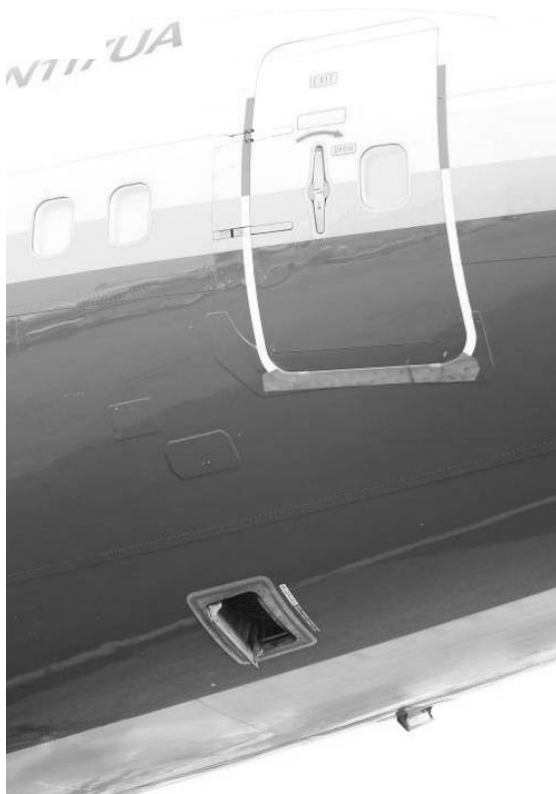
(a) patches surrounding door
