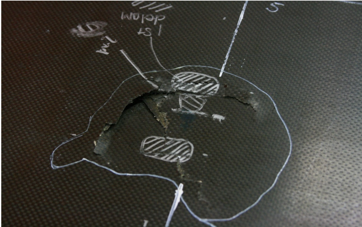
Figure 23. Stringer01 skin penetration and delamination damage
