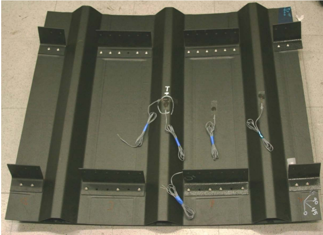
Figure 10. Stringer focused test specimen (series ID: StringerXX); 2-stringer panel not shown would be impacted on skin between stringers
