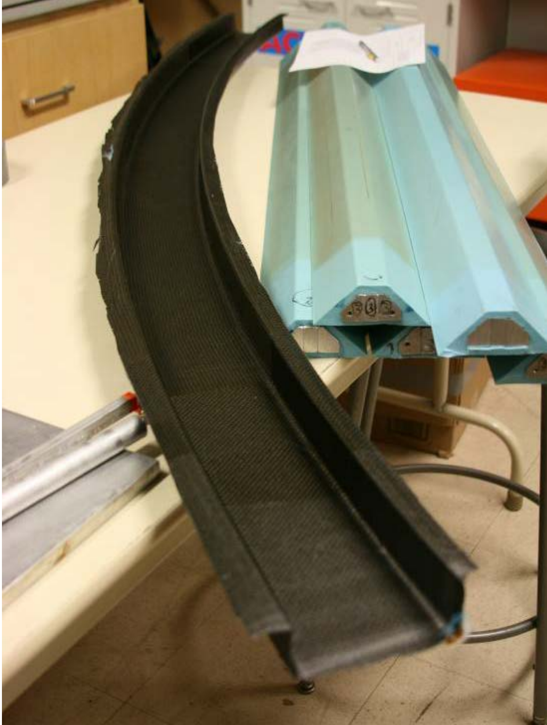
Figure 18. Untrimmed C-frame; stringer internal silicone molds
