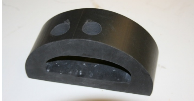
Figure 14. OEM rubber bumper for stringer specimen tests
