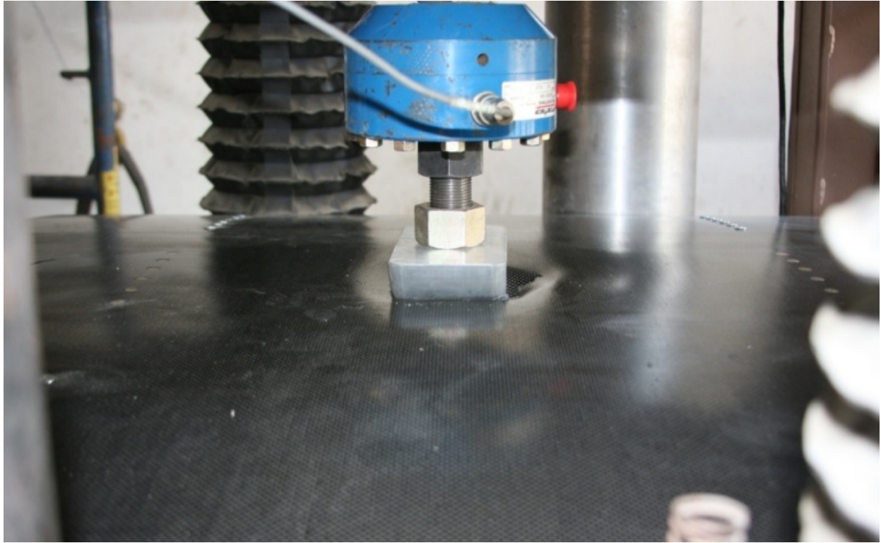
Figure 22. Stringer01 local skin penetration
