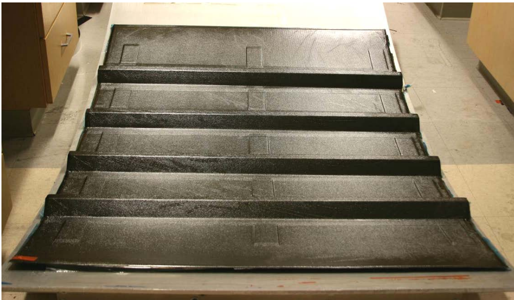
Figure 16. Three-frame specimen without frames or shear ties; approximate overall dimensions 1.83 m in curved direction by 1.2 m in stringer direction
