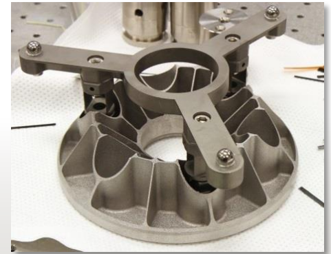
prototype AM mirror & structure
