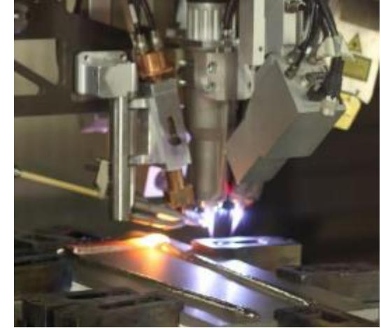
Part deposition in MERKE IV™ RPD™ Machine Picture courtesy of Norsk Titanium
