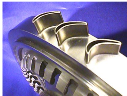
Building airfoils on turbine disc to form a “blisk”.
