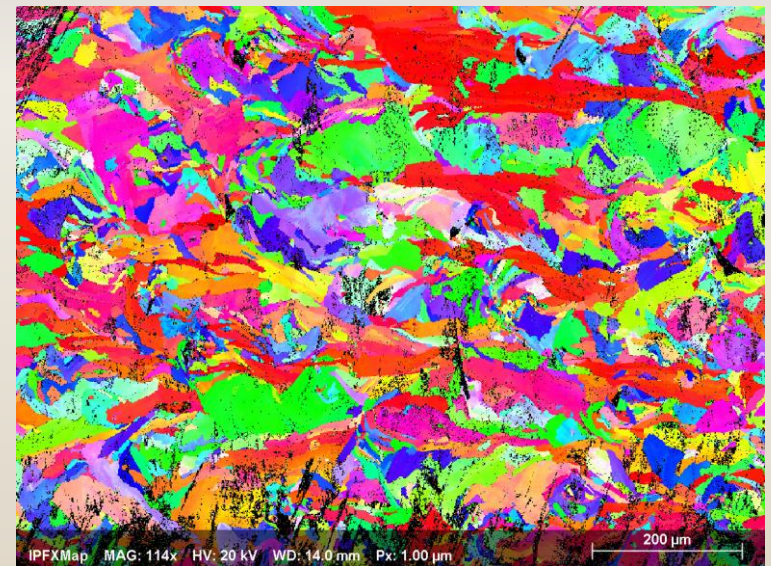
representative texture map via EBSD, phase content has been relatively consistent across process settings
