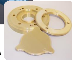
Paint Masks for Engine Housings
