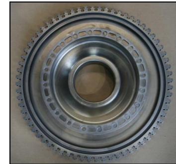
Build/repair of IN718 with laser system – process development and optimization (high mechanical properties at elevated temperatures in service) to demonstrate repair of heavily damaged turbine rotors
