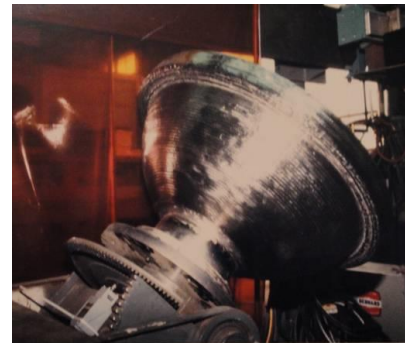
Nuclear component Using GTAW-P
