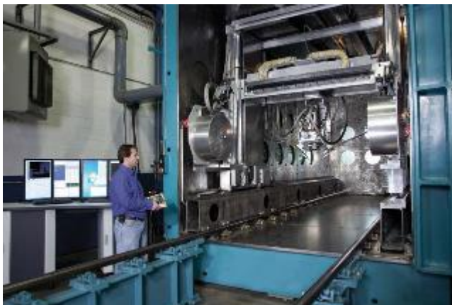
Electron Beam Additive Manufacturing (EBAM™) Machine Picture courtesy of Sciaky
