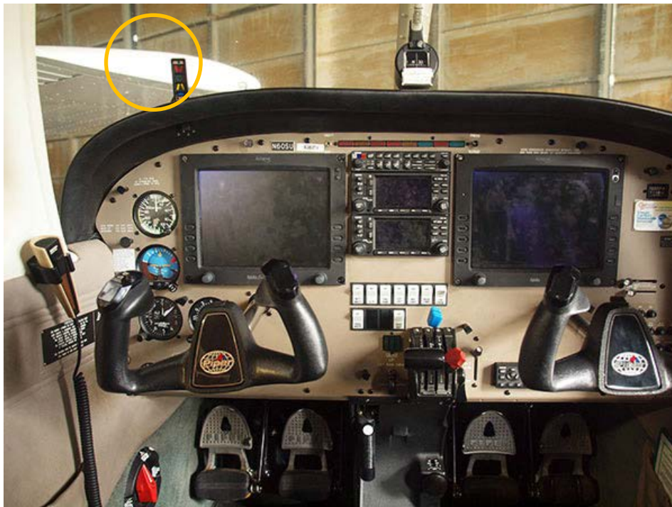
Figure 3. AOA display installed in Piper Arrow and Warrior aircraft
