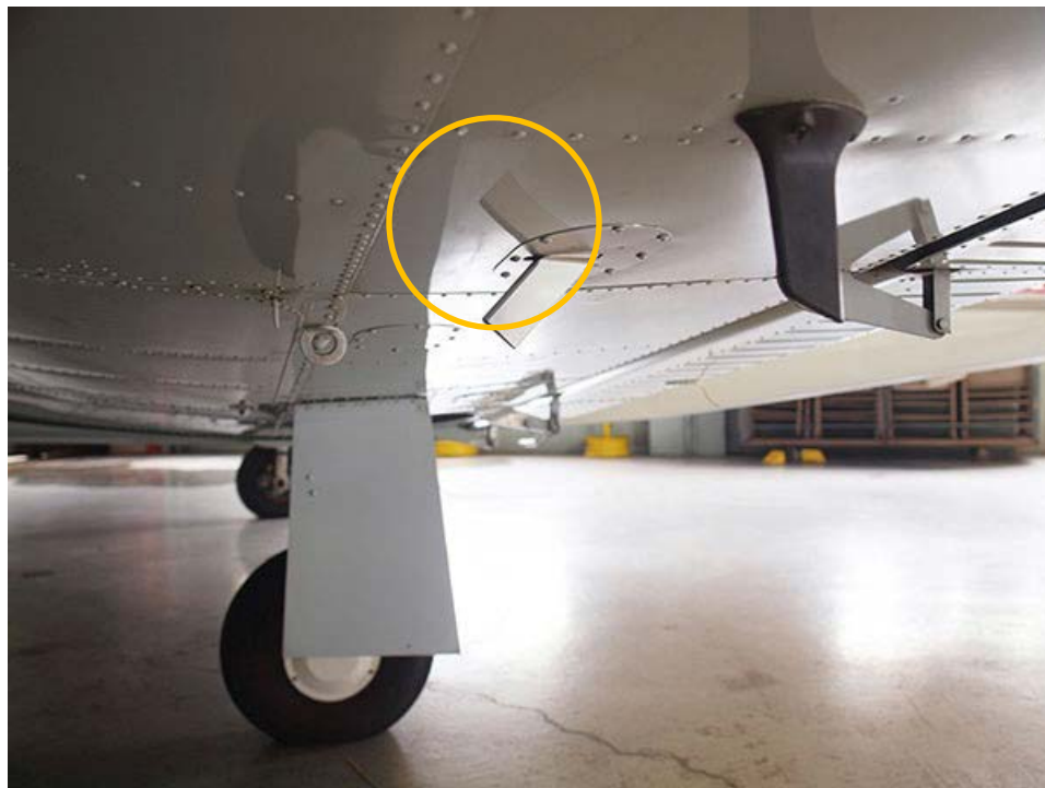
Figure 4. AOA probe on Piper Arrow aircraft
