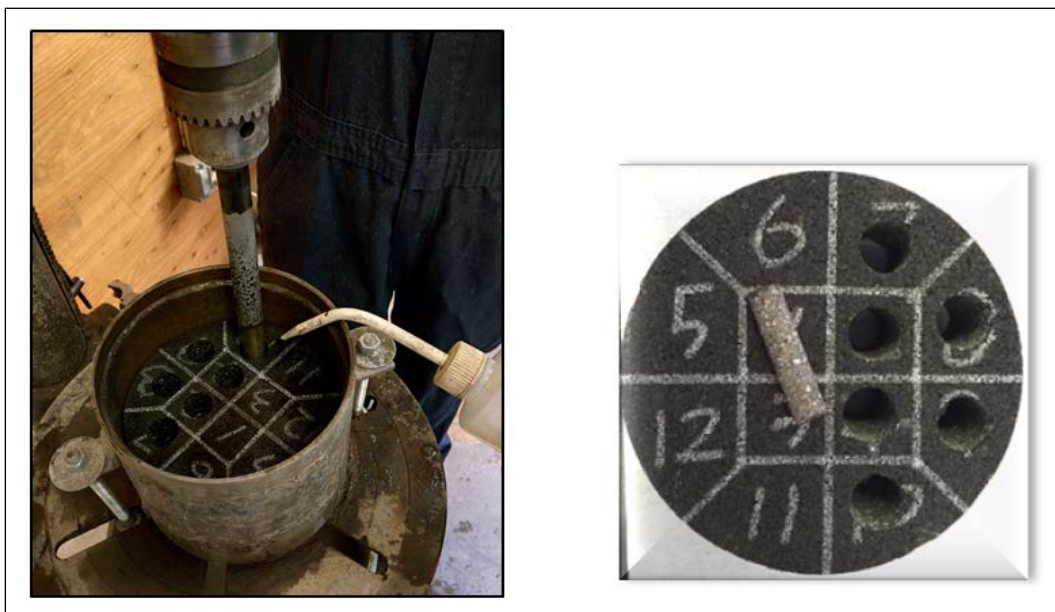
Figure 7. The FAM Mix Specimens Cored From a Superpave Gyratory-Compacted Specimen
