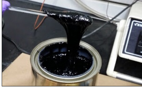
Figure 4. Recovered RAS Binder After 3 Hours of Conditioning at 190°C
