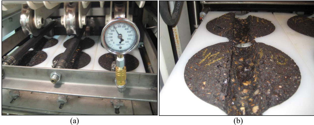
Figure 5. The APA Test Configuration (a) and HMA Specimens After Testing in the APA (b)
