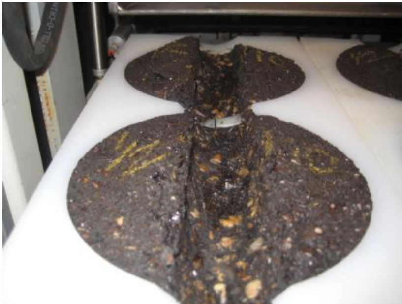
Figure 6. The HMA Specimens After Testing in the APA
