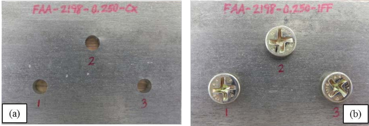
Figure 3. Fastener hole processing specimens: Al-Li 2198-T8; 0.25" thick; (a) cold expansion; (b) interference fit fasteners
