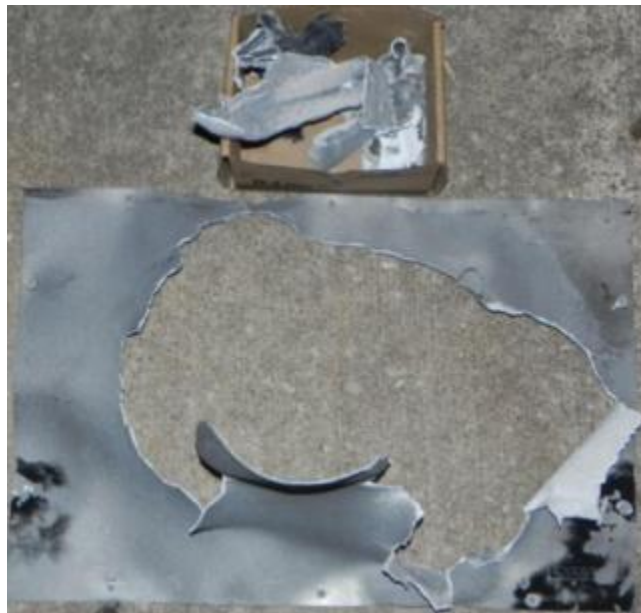
Figure 6. Flammability result: 0.071" Al-Li 2198-T8 specimen post test
