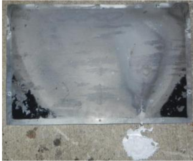
Figure 7. Flammability result: 0.125" Al-Li 2198-T8 specimen posttest
