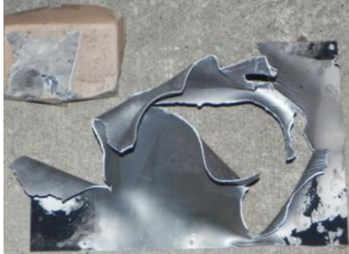
Figure 5. Flammability result: 0.125" AA 2024-T3 specimen post test
