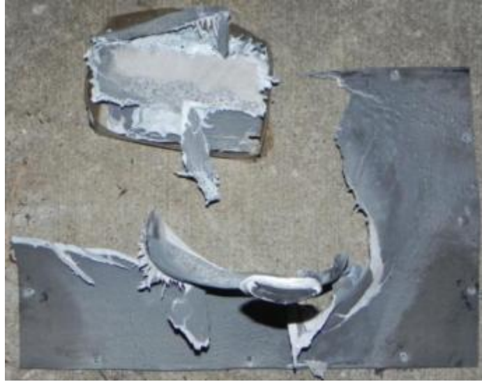
Figure 8. Flammability result: 0.25" Al-Li 2198-T8 specimen post test
