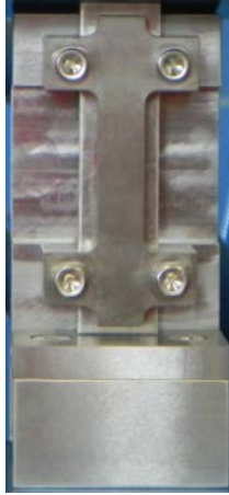
Figure 10. FAA WJHTC anti-buckling jig
