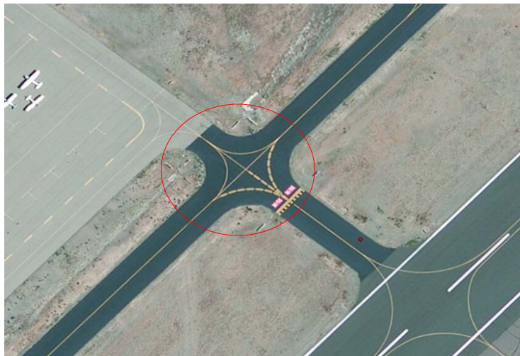
Figure 18. Short Taxi Distance to Runway From an Apron
