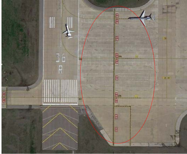
Figure 14. Nonstandard Marking Placement
