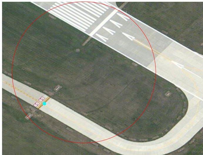
Figure 22. Displaced Threshold With Holding Position Marking on Parallel Taxiway
