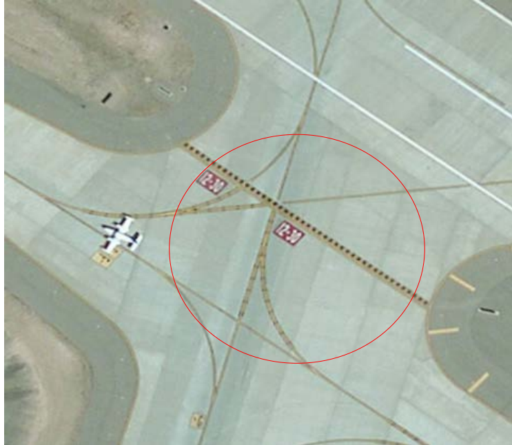
Figure 8. Converging Taxiway Types for a Runway
