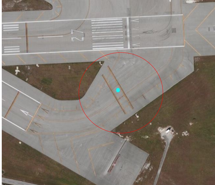
Figure 10. Runway Thresholds in Close Proximity
