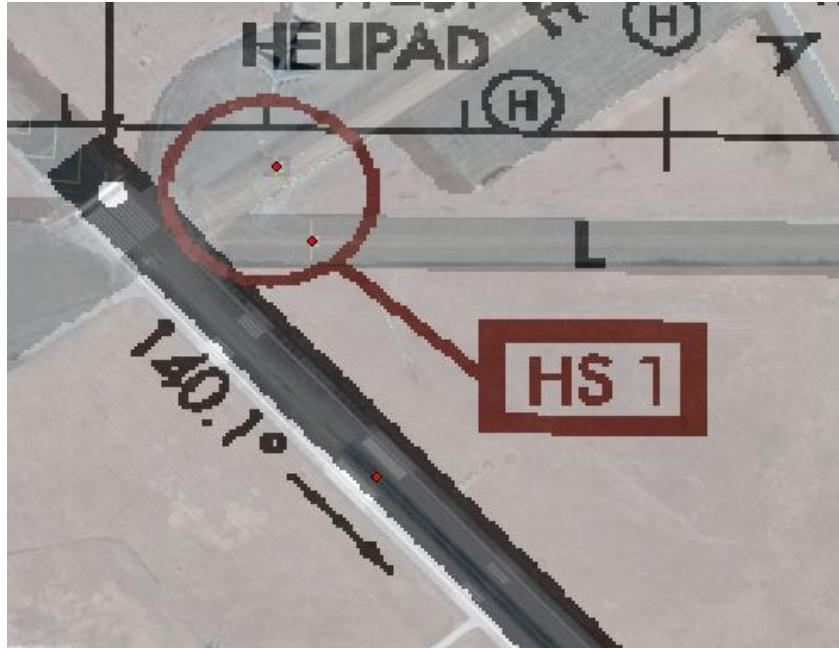
Figure 3. Hot Spot Depiction on Airport Diagram
