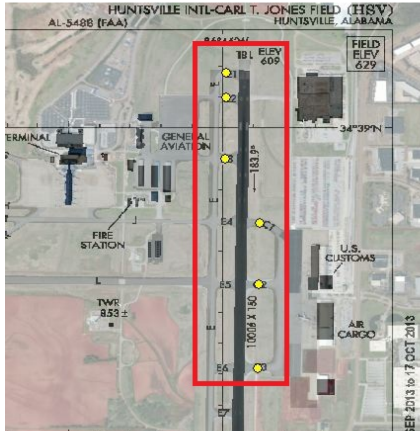
Figure 4. Problematic Taxiway Geometry Locations
