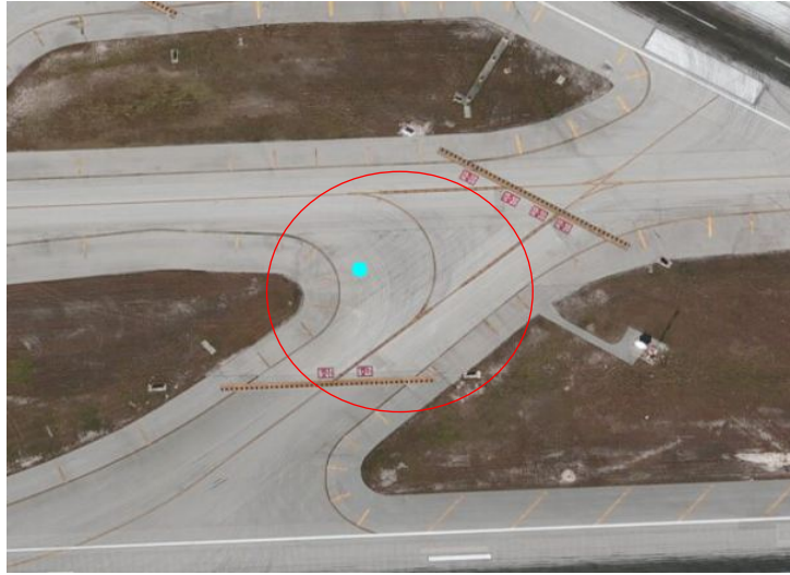
Figure 19. High-Speed Exit Leading Directly to Another Runway
