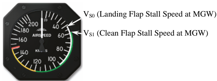
Figure 1. Conventional airspeed indicator LSA markings
