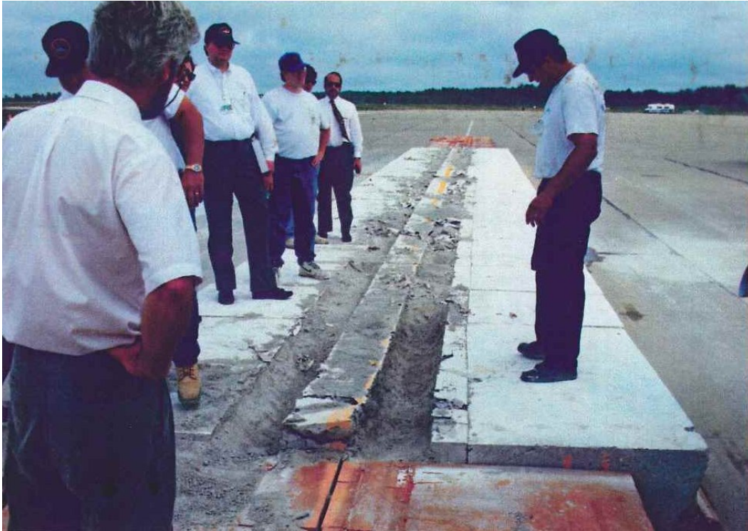
Figure 6. The B-727 Nose Gear Ruts
