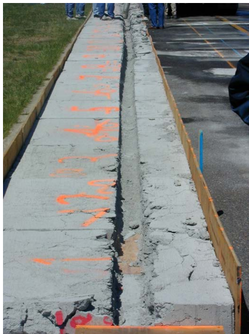
Figure 45. Wheel Ruts From the Small-Wheel Test Through the Non-JBR Blocks
