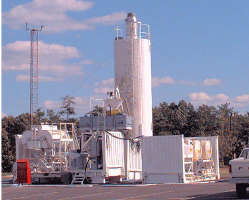
Figure 8. The ESCO Cellular Cement Block Manufacturing Plant at WJHTC
