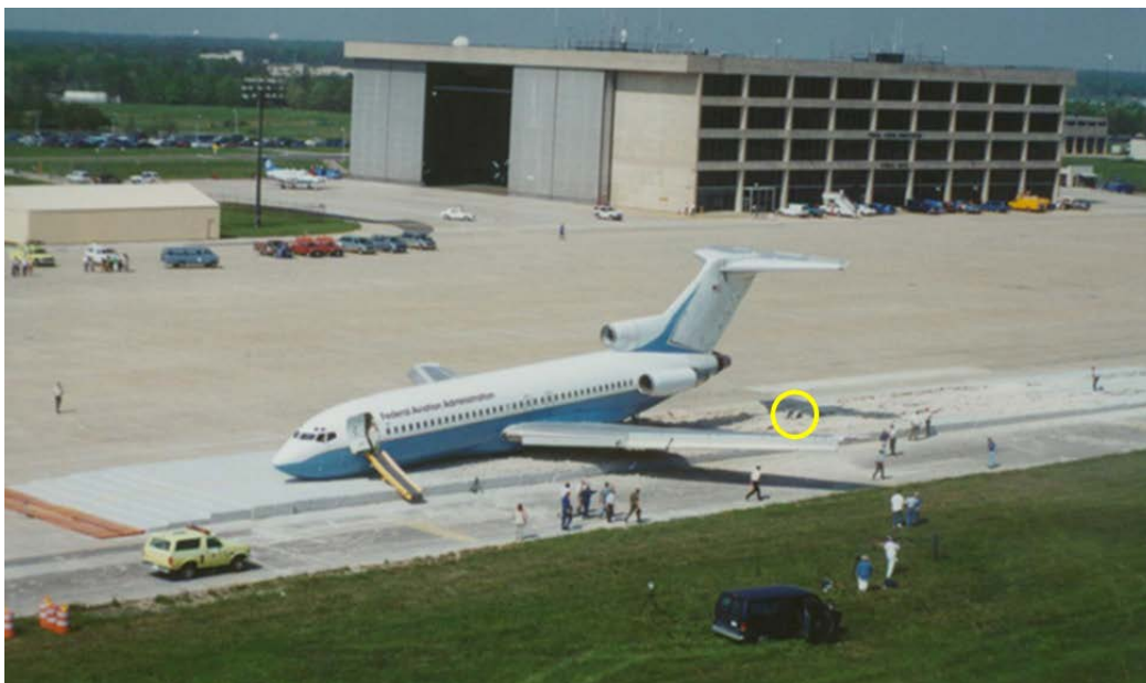
Figure 12. The B-727 Stopped 278 ft Into the Cellular Cement Test Bed
