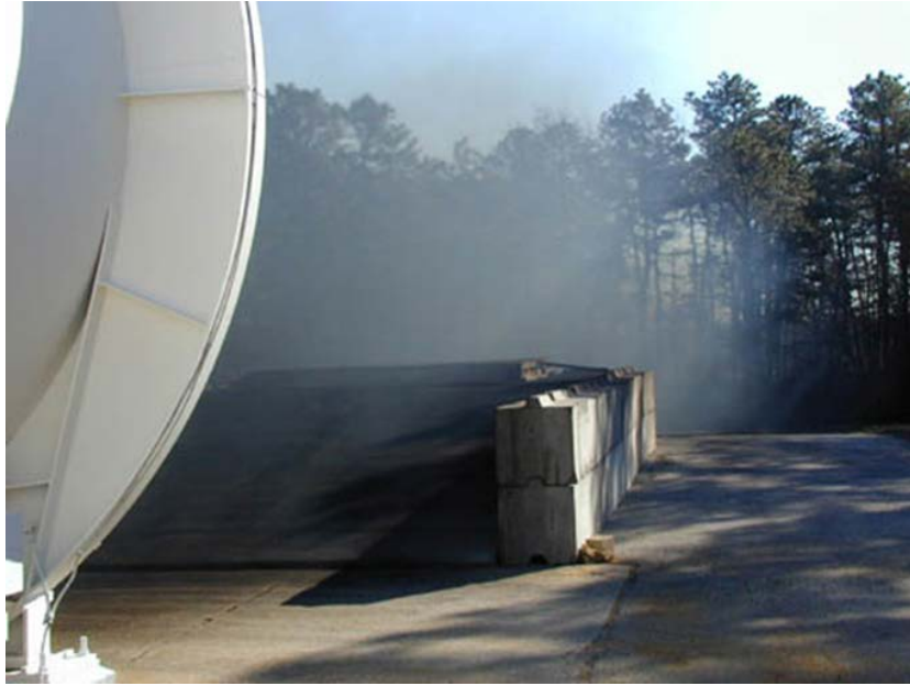
Figure 34. Wind Tunnel Jet Blast at 100% Rated Speed
