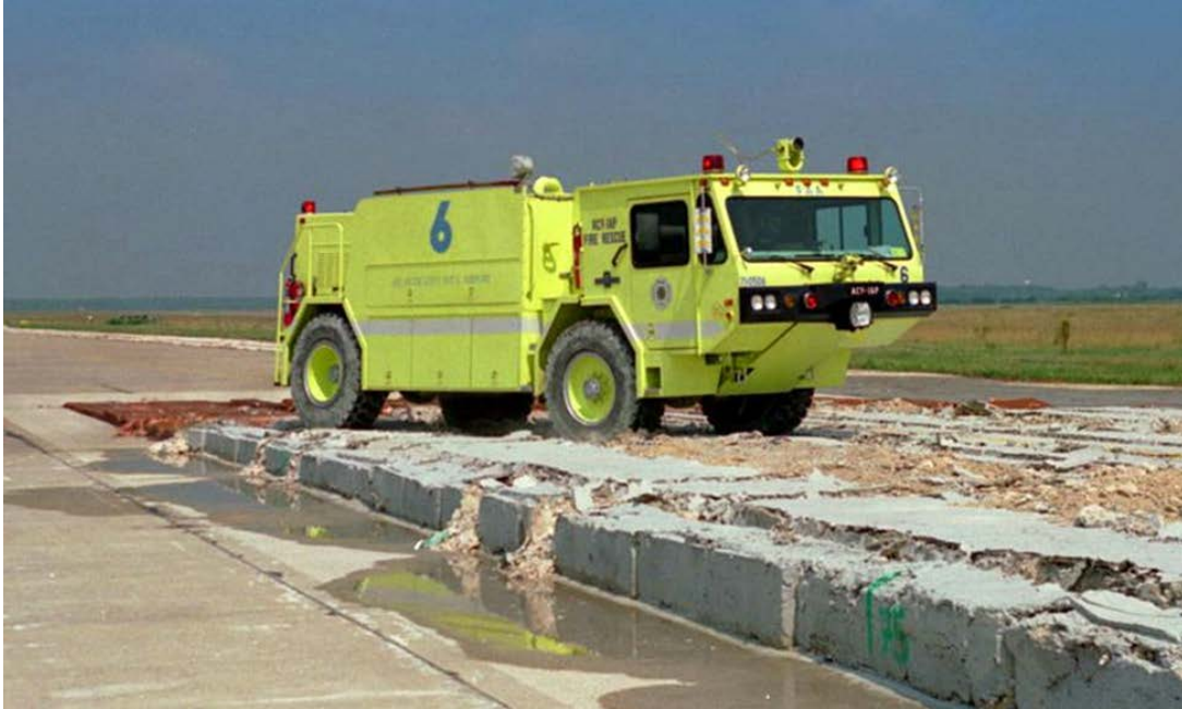
Figure 19. The P-19 ARFF Vehicle Maneuvering in Arrestor Bed
