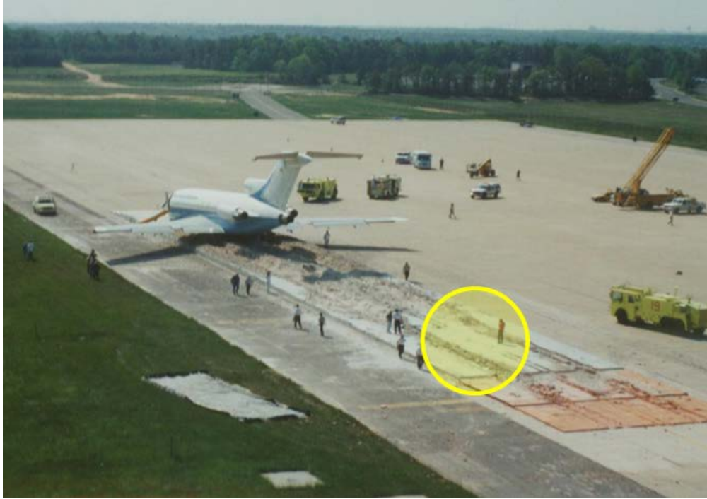
Figure 11. Area Highlighted Shows Where Nose Gear Lifted From Test Bed
