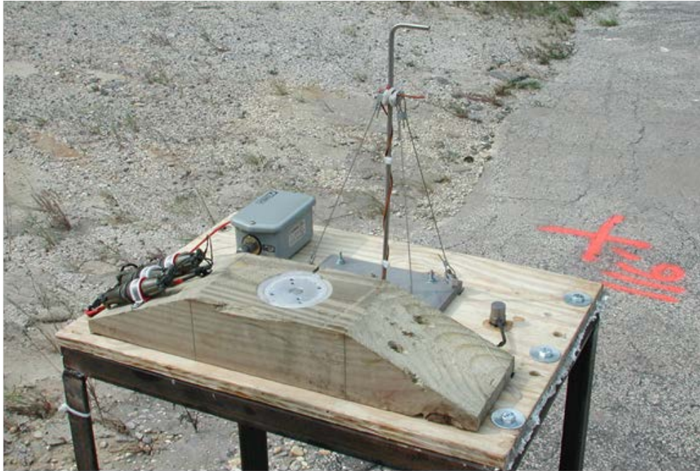
Figure 28. Instrumentation Package Mounted on a 36-in.-High Metal Stand Behind the Wind Tunnel
