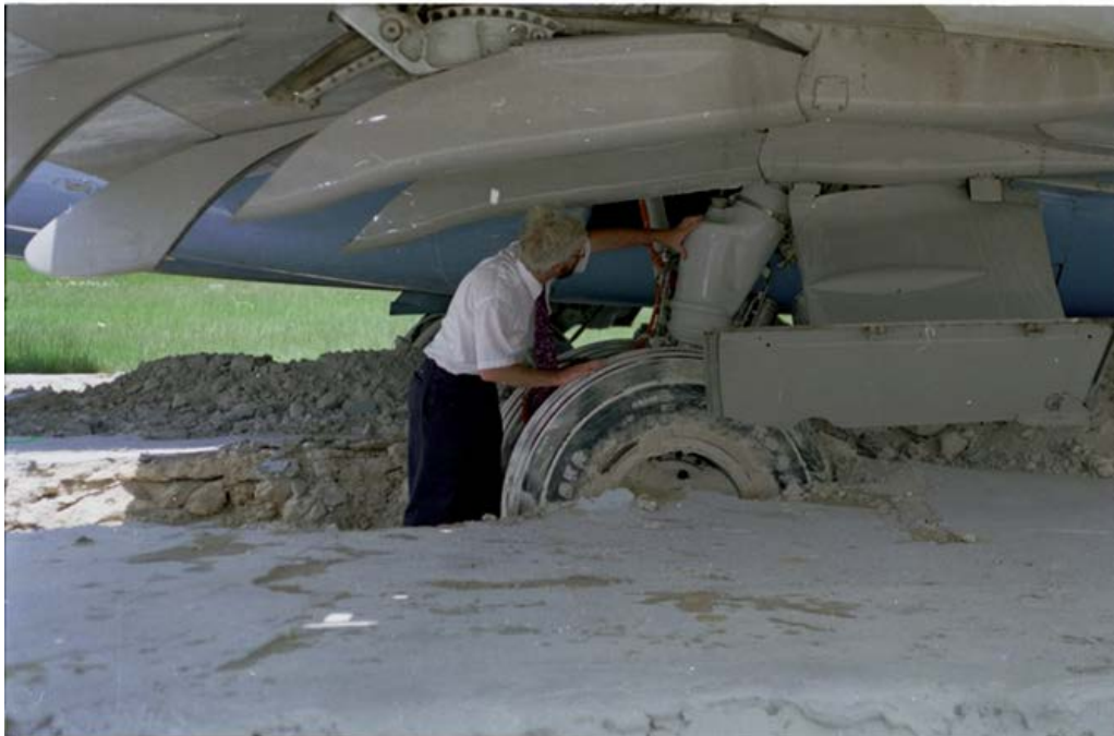
Figure 17. Right Main Gear Inside the Cellular Cement Test Bed
