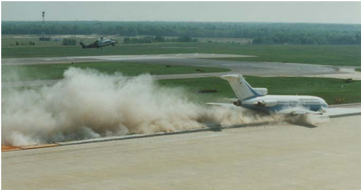
Figure 10. The B-727 Entering Cellular Cement Test Bed at 55 kt
