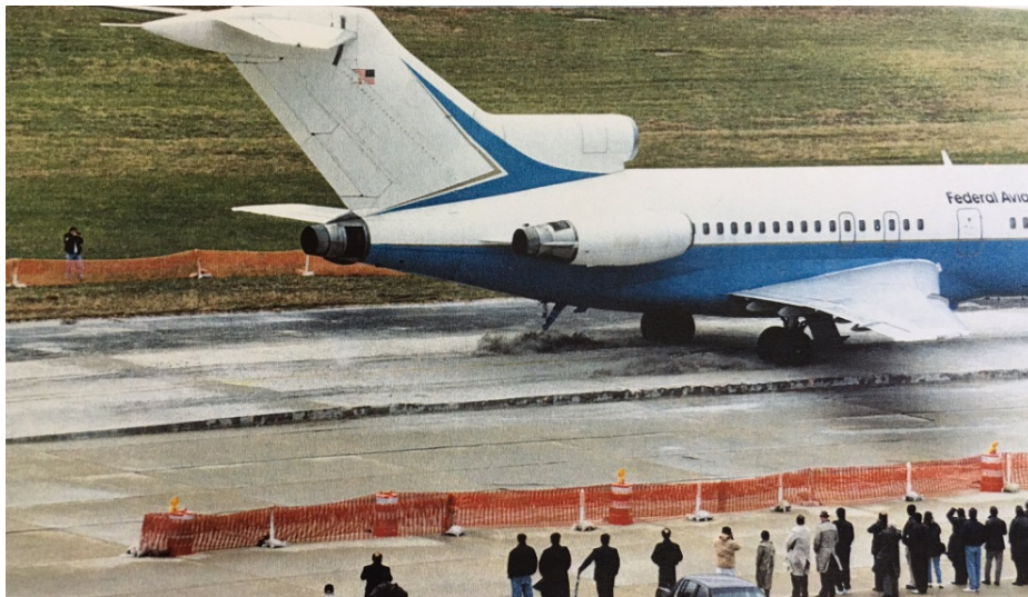
Figure 3. The FAA B-727 Aircraft Entering Foamed Concrete Test Bed at the WJHTC
