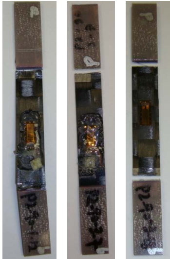
Figure A-20. Failure modes for Toray [90°] 4 at stroke rate of 2 in/s
