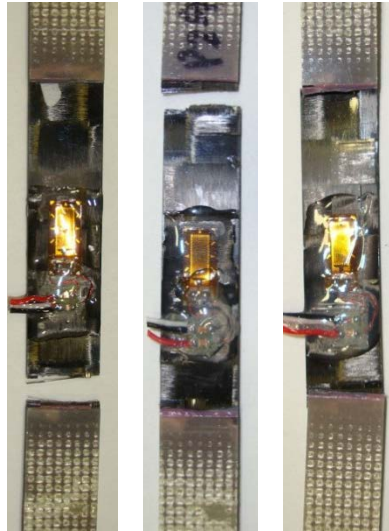
Figure F-5. Failure modes for Toray [90°] 4 at stroke rate of 0.00083 in/s
