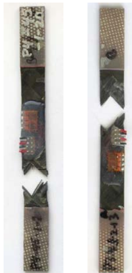
Figure C-17. Failure modes for Toray [ \pm 45^\circ ] 4 at stroke rate of 0.02 in/s
