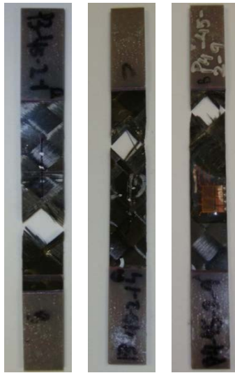
Figure A-28. Failure modes for Toray [ \pm 45^\circ ] 4 at stroke rate of 2 in/s
