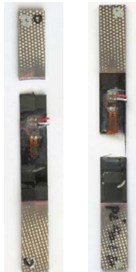
Figure C-9. Failure modes for Toray [90°] 4 at stroke rate of 0.02 in/s
