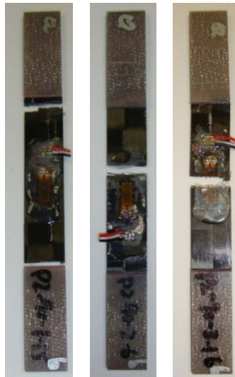
Figure A-24. Failure modes for Toray [90°] 4 at stroke rate of 500 in/s
