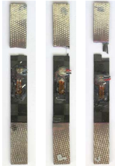
Figure C-15. Failure modes for Toray [90°] 4 at stroke rate of 500 in/s
