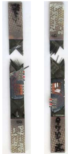
Figure C-19. Failure modes for Toray [ \pm 45^\circ ] 4 at stroke rate of 2 in/s
