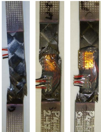
Figure F-7. Failure modes for Toray [ \pm 45^\circ ] 4 at stroke rate of 0.00083 in/s
