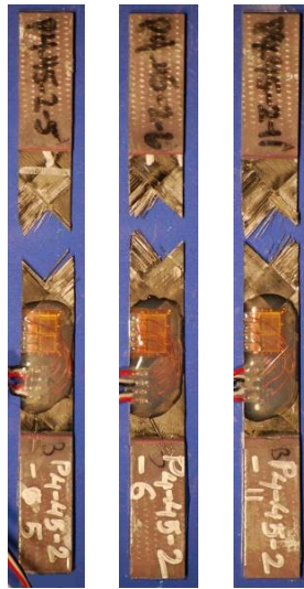
Figure B-17. Failure modes for Toray [\pm 45^\circ]_4 at stroke rate of 200 in/s
