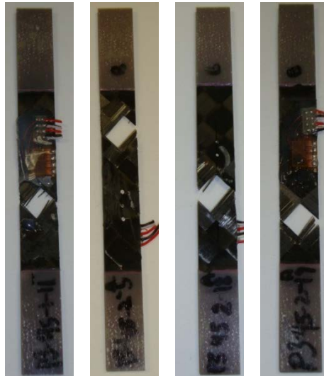
Figure A-30. Failure modes for Toray [ \pm 45^\circ ] 4 at stroke rate of 200 in/s
