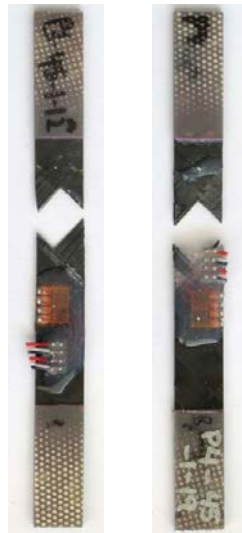
Figure C-21. Failure modes for Toray [ \pm 45^\circ ] 4 at stroke rate of 200 in/s
