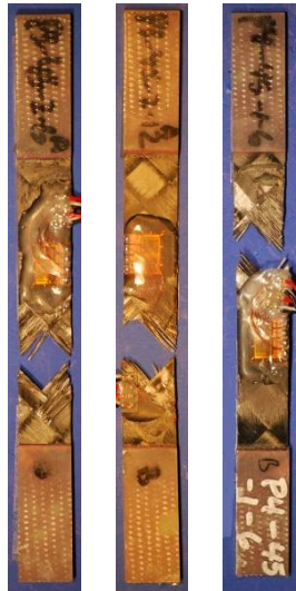
Figure B-13. Failure modes for Toray [ \pm 45^\circ ] 4 at stroke rate of 0.02 in/s
