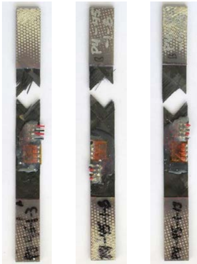
Figure C-23. Failure modes for Toray [ \pm 45^\circ ] 4 at stroke rate of 500 in/s
