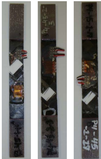
Figure A-32. Failure modes for Toray [ \pm 45^\circ ] 4 at stroke rate of 500 in/s
