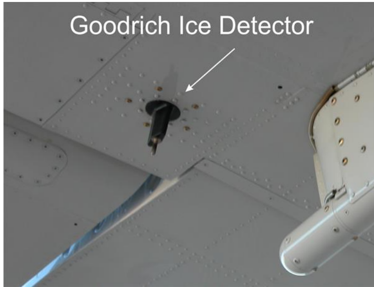
Figure 22. Goodrich Ice Detector under the wing of the NRC Convair-580 aircraft
