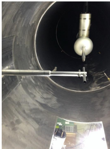
Figure B-4. ICTs installed on mast ahead of the IKP-22, at the NRC M7 open-cell wind tunnel [B-1]
