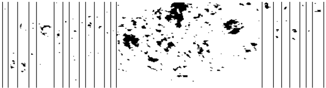
Figure C-3. Example of shattering event (largest image near center of frame) as recorded by the 2D-S probe
