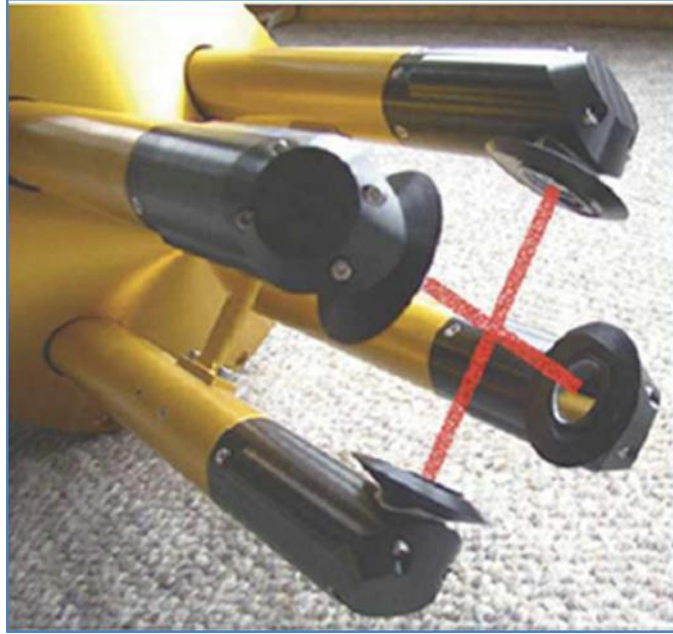
Figure 18. Forward sampling arms of the SPEC 2D-S probe with simulated projection of the laser sample volume of the two independent probes ([43])
