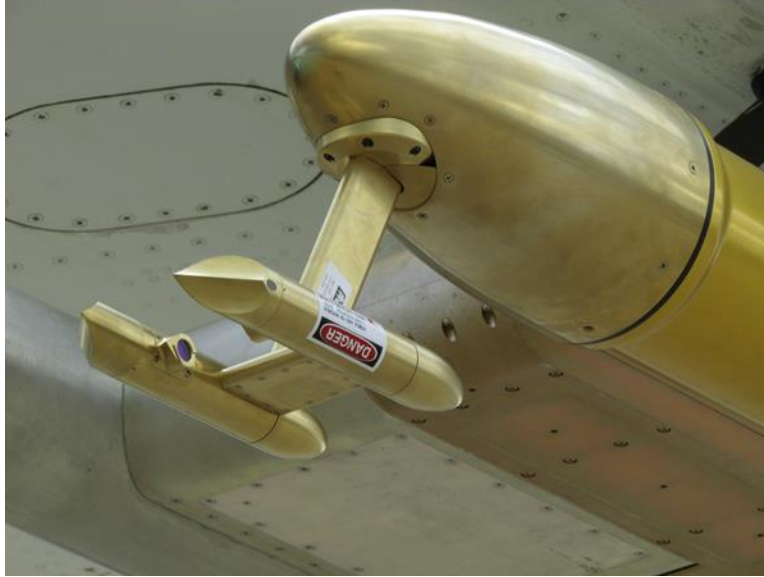
Figure 17. DMT CDP-2 under the wing of the NASA DC-8 aircraft during the HIWC RADAR flight campaign
