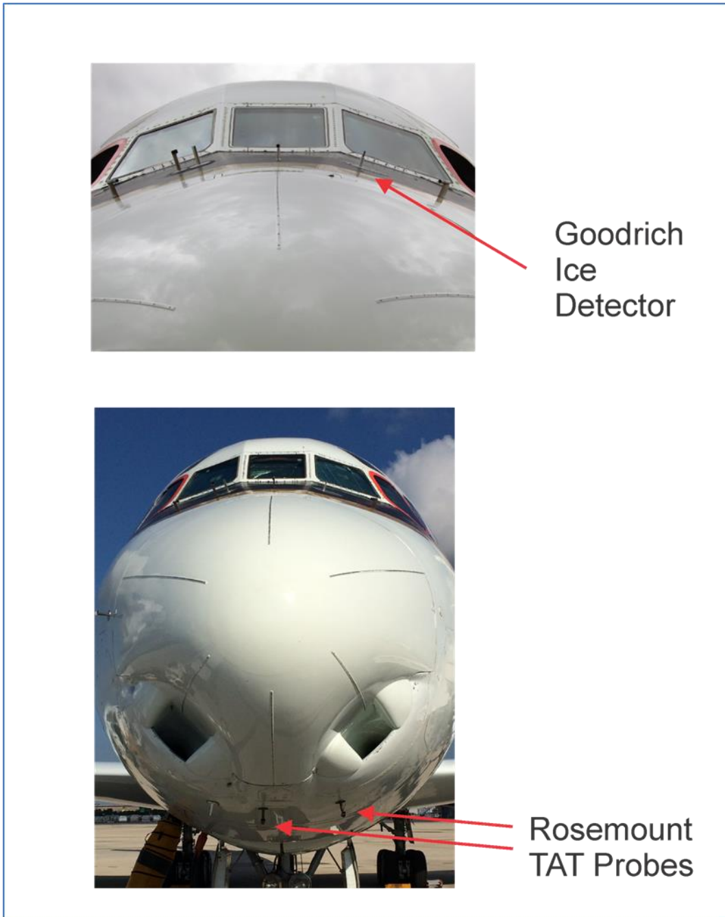
Figure 26. Location of probes on the DC-8 during the HIWC-RADAR Florida-15 flight campaign
