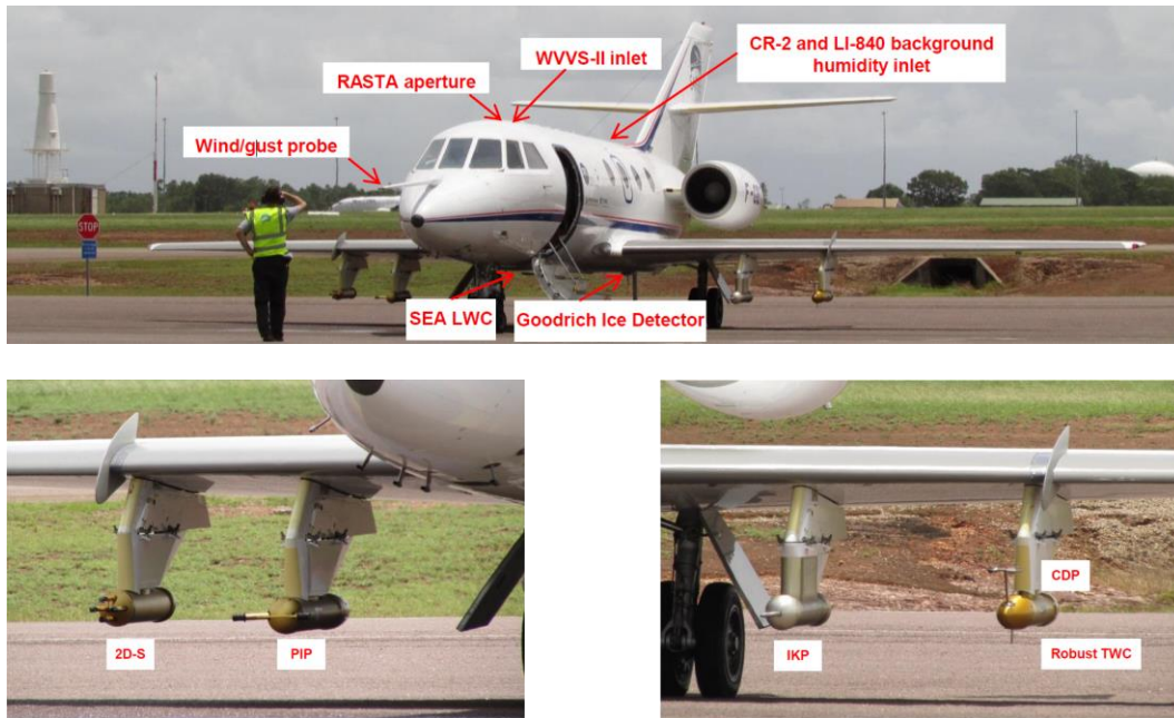
Figure 23. Location of primary probes on the Falcon-20 during the HAIC-HIWC Darwin-14 and Cayenne-15 flight campaigns
