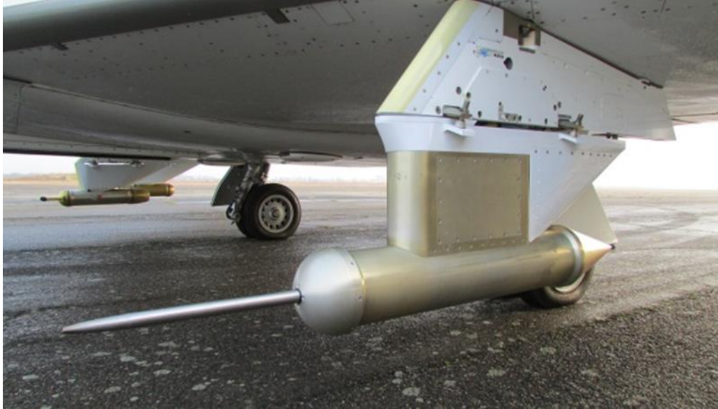
Figure 11. Isokinetic evaporator (IKP-2) under the wing of the Falcon-20 aircraft ([38])
