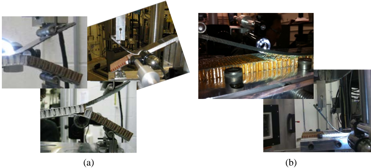
Figure 3. The (a) DCB and (b) SCB test configurations [9]
