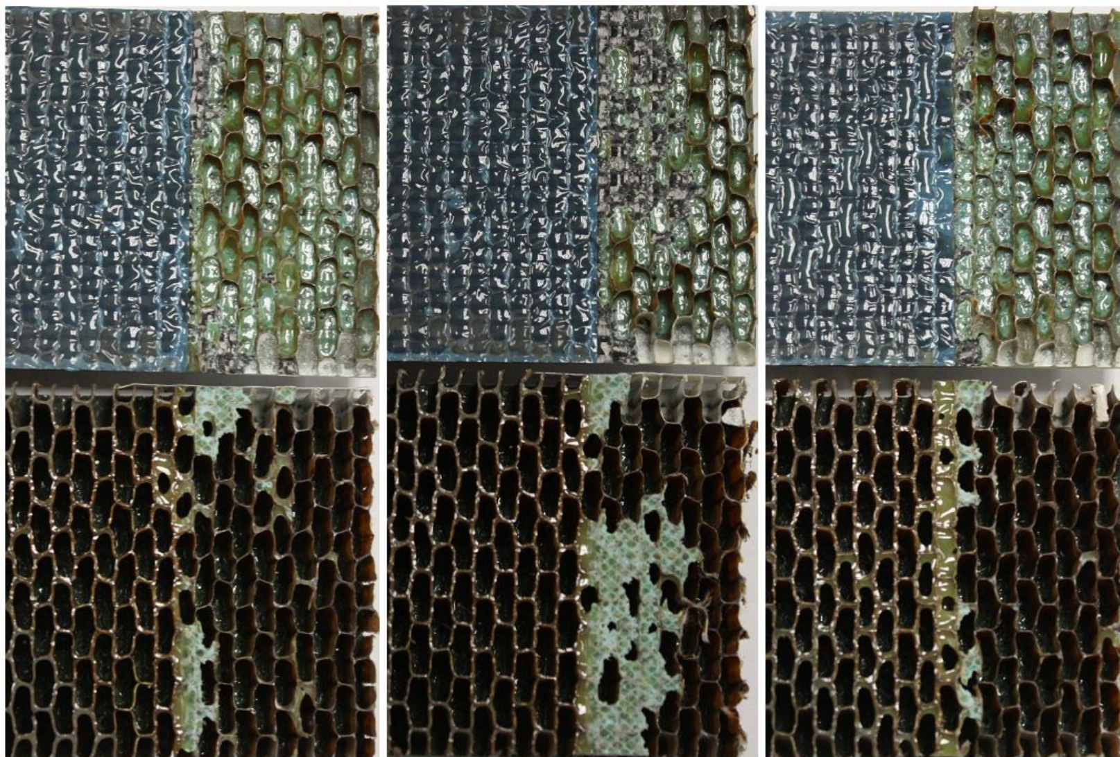
Figure D-4. Failure mode image of SDT-04-OX-13.16-3-BL-SLX-X (shortened) #5, #6, and #8
