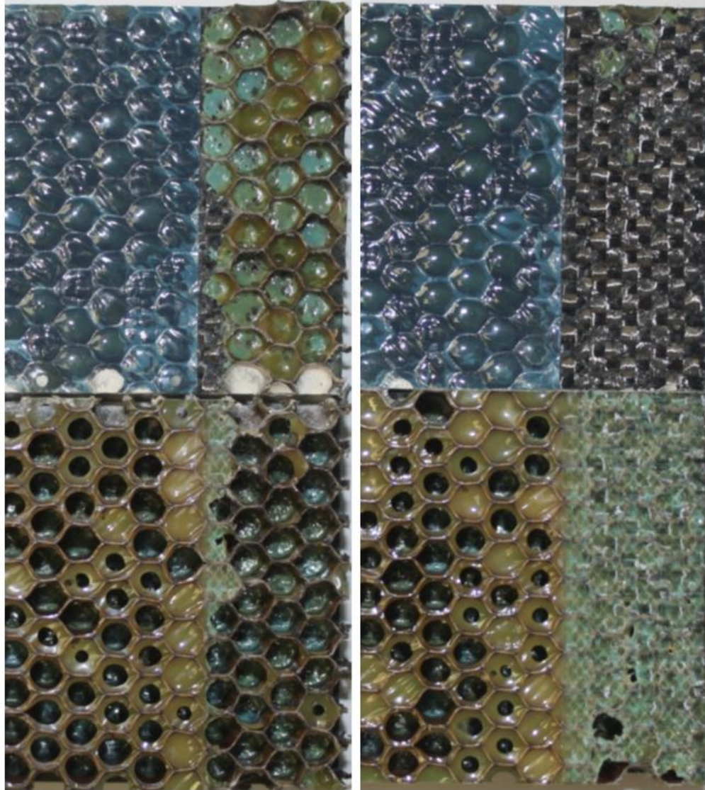
Figure C-40. Failure mode image for SDT-16-HX-3.16-6-FI-SLX-X #1** and #2**
