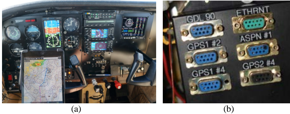
Figure 13. N736WP instrument panel (a) and data connections under panel (b)
