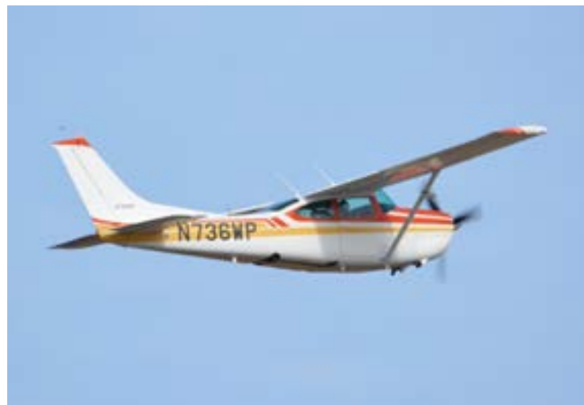
Figure 12. N736WP is a 1979 Cessna R182 equipped to obtain calibrated ADAHRS and angle-of-attack data
