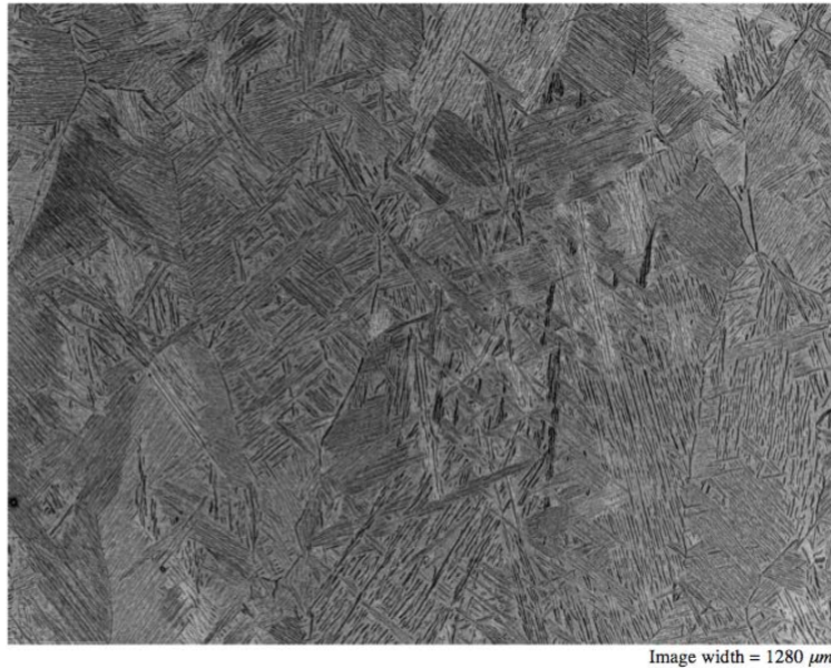
Figure 5. Microstructure of Ti-6242 Pancake 3 in the AR condition
