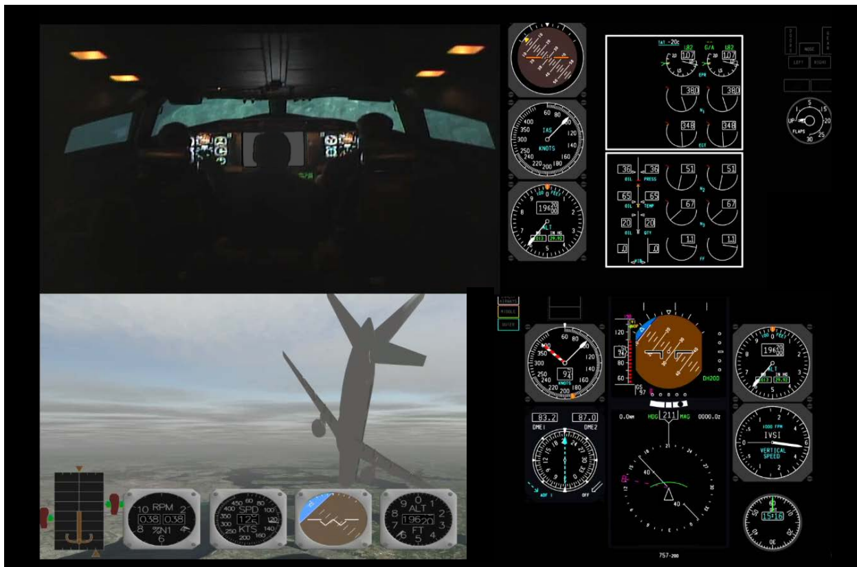
Figure 13. Pilot-in-the-loop simulations in multipurpose cab (M-Cab) at Boeing
