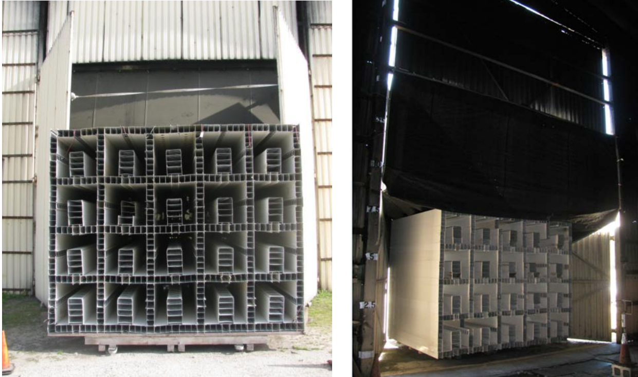
Figure 6. Air Entrance Into Hangar Through Flow Straightener
