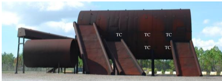
Figure 11. Surface-Mounted TC Locations on the Right Side of the Full-Scale NLA Mockup
